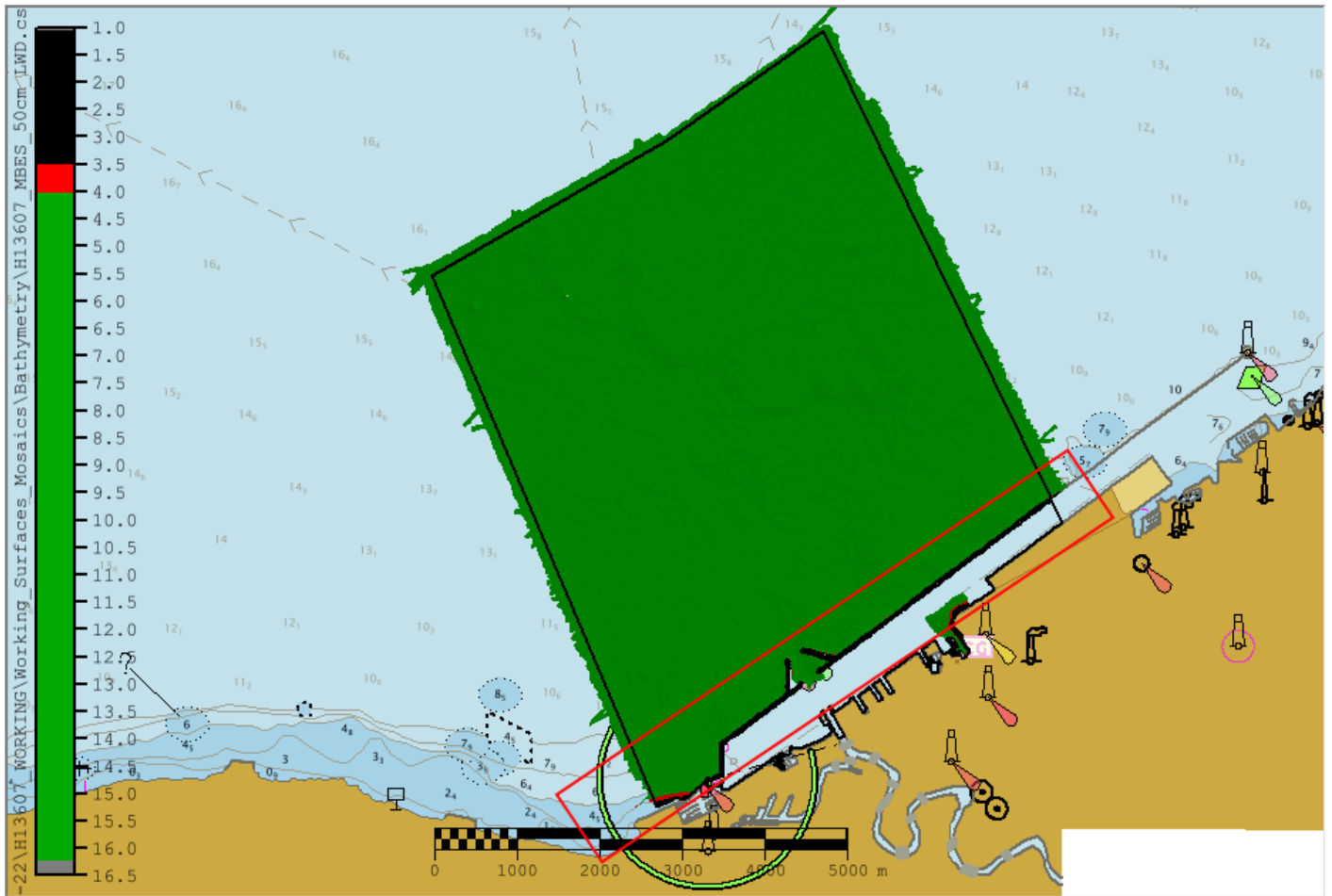
Figure 3: Areas where coverage did not meet 3.5m depth contour for the assigned sheet limits was mostly along the breakwater outlined in red.
