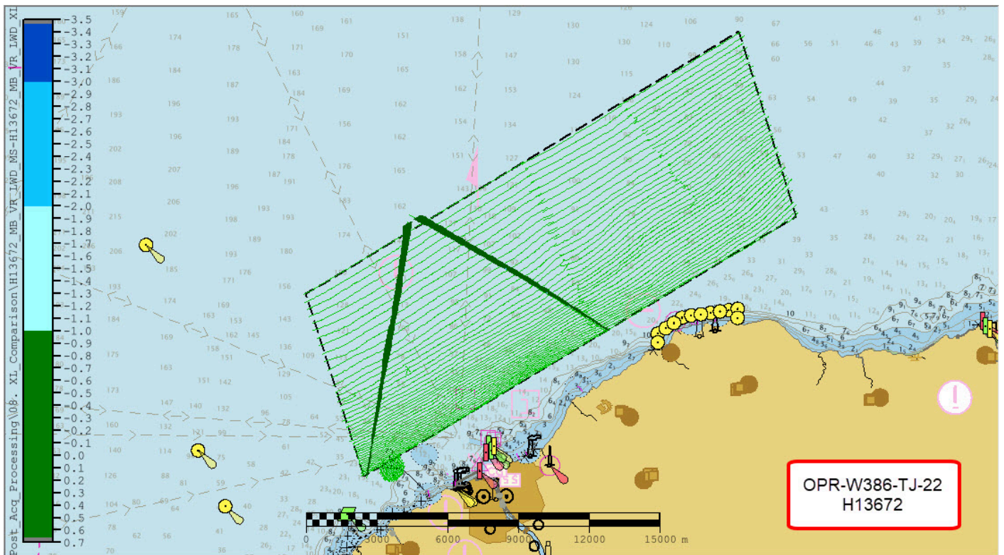
Figure 6: An overview of H13672's crosslines overlaid on the survey tracklines and ENC US4NY22M showing good spatial distribution
