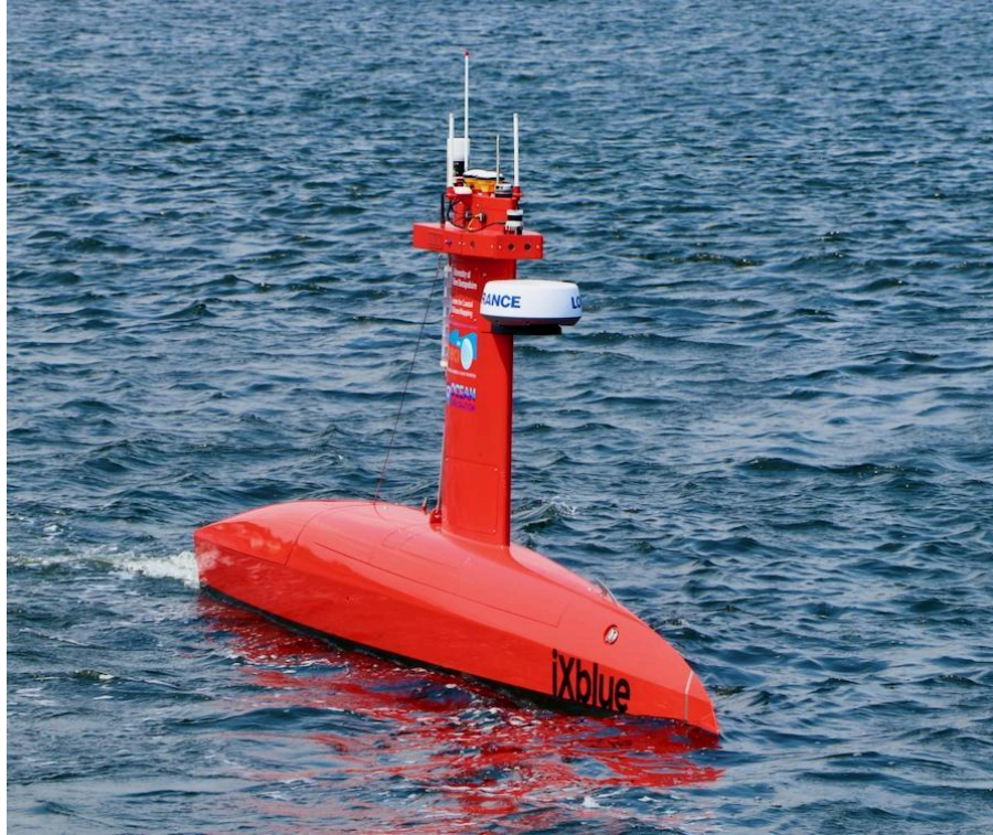
Figure 5: Autonomous Survey Vehicle DriX-12
