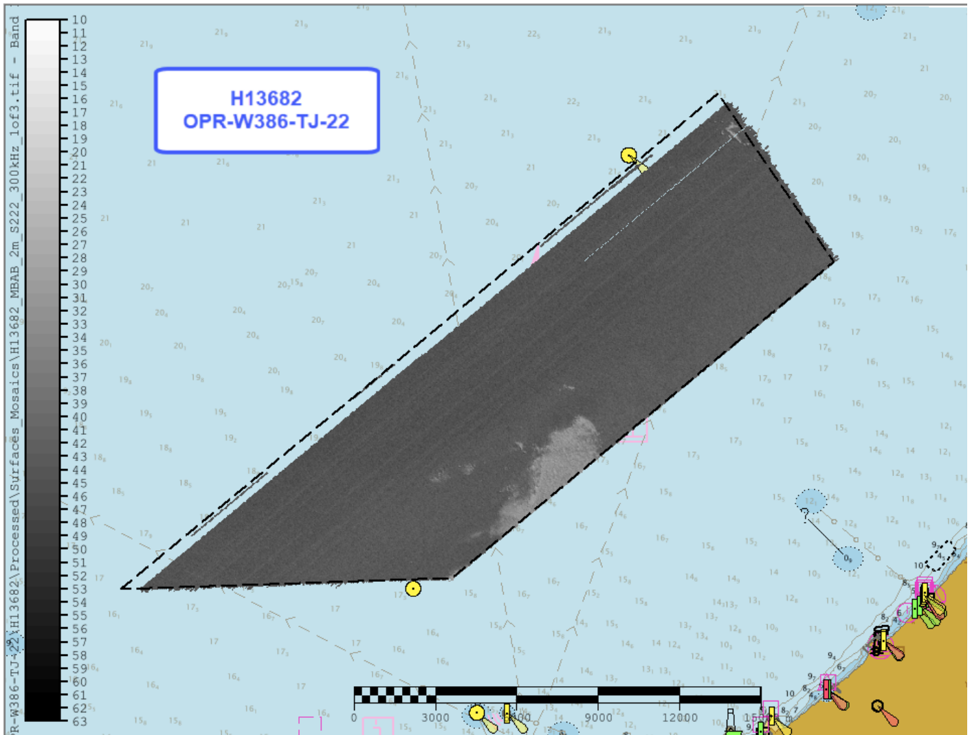
Figure 20: 300kHz backscatter mosaic from data acquired by S-222.
