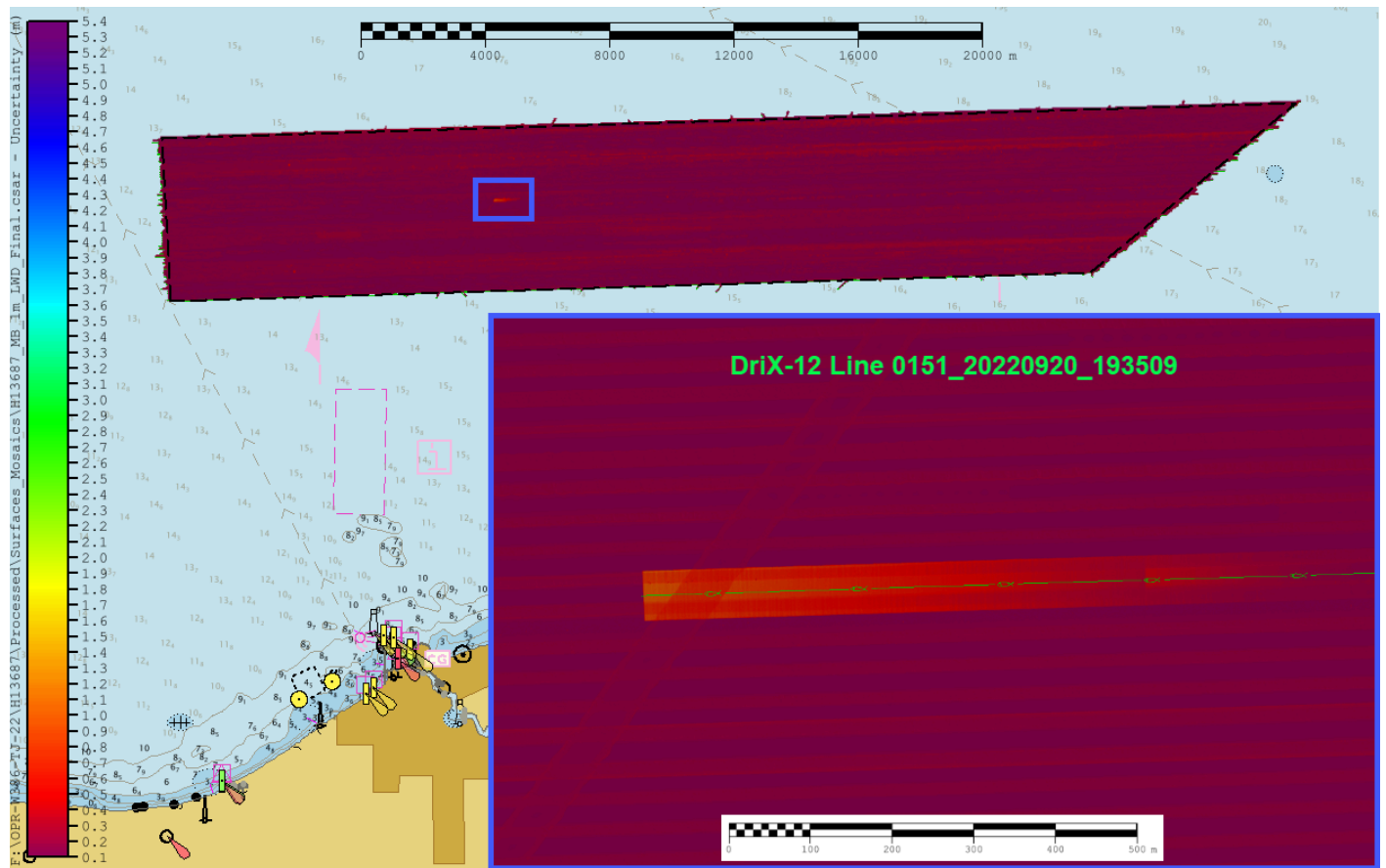
Figure 10: DriX-12 line showing increased uncertainty values of up to 1m.
