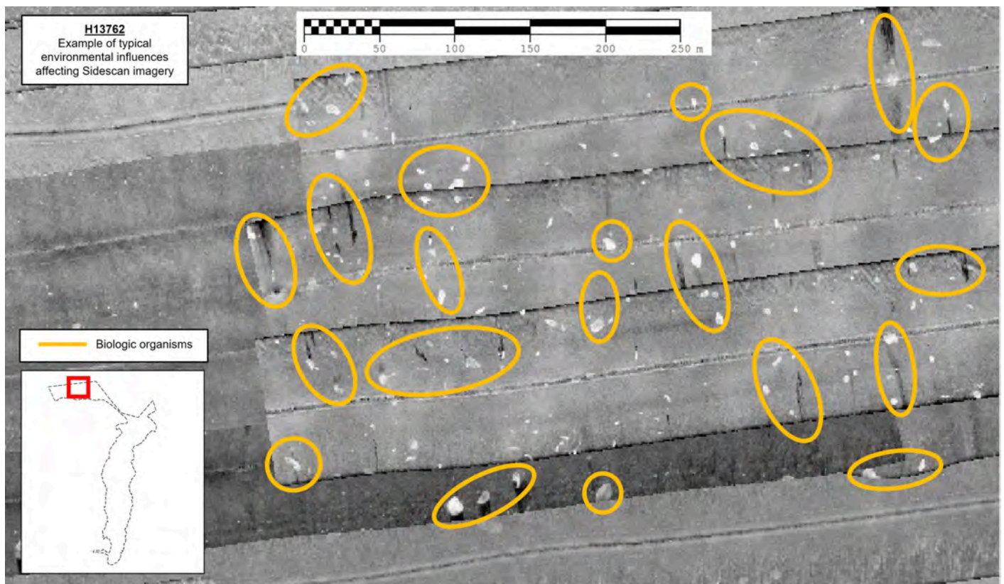
Figure 17: Example of environmental influences affecting SSS imagery which were persistent throughout the survey area, present within the final delivered mosaic.
