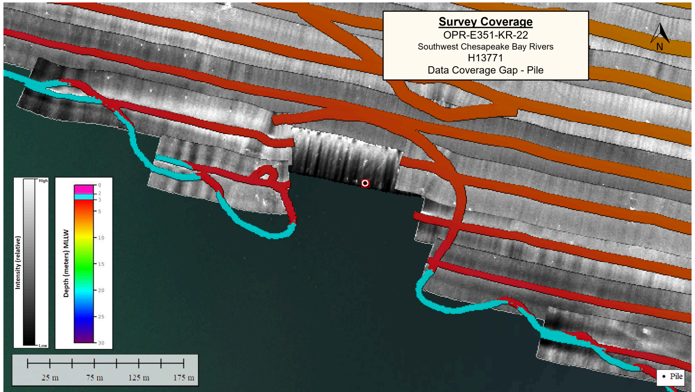
Figure 5: Data coverage gap caused by piles
