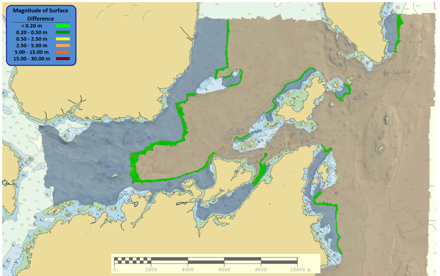
Figure 14: Difference surface between H13776 (grey) and junctioning survey H13407 (brown).
