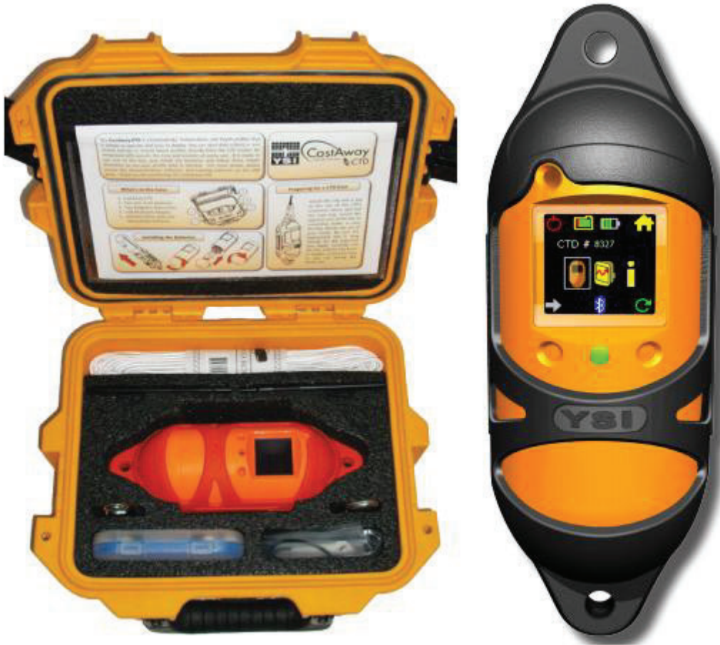
Figure 10: Castaway Sound Speed Sensor used aboard S3008 and S3005
