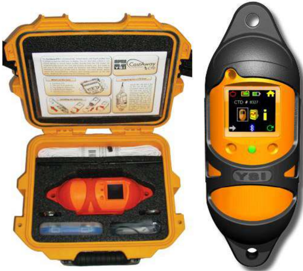
Figure 8: Castaway Sound Speed Sensor used aboard S3008
