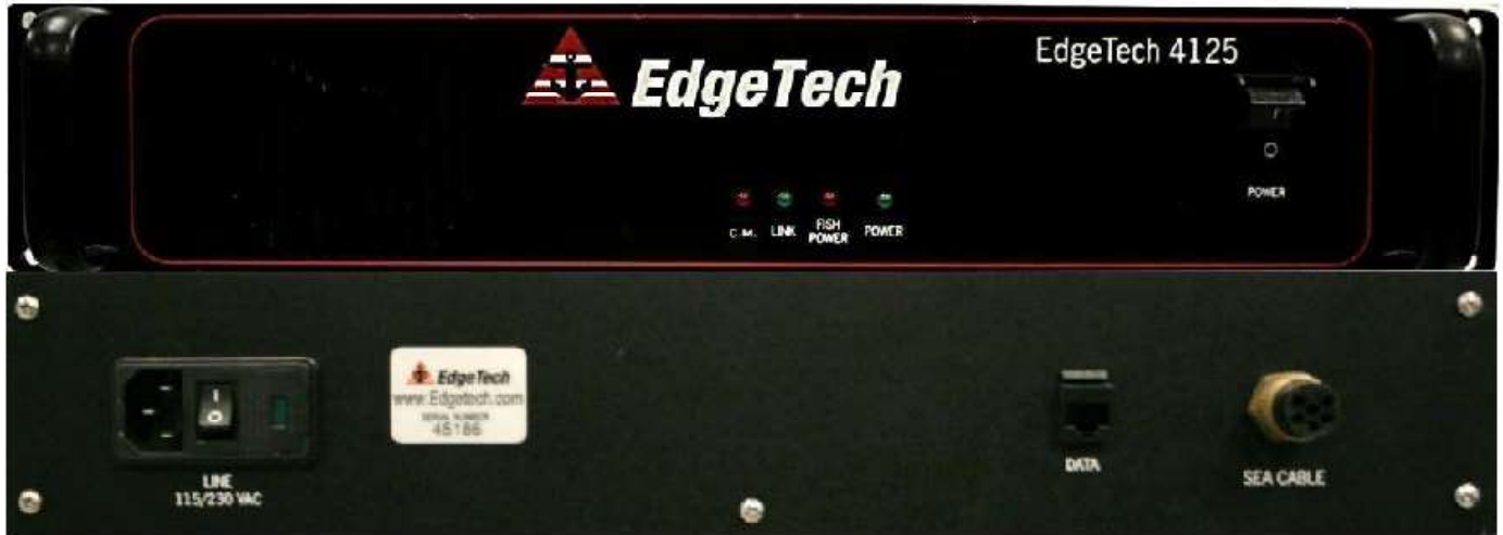
Figure 7: Edgetech 4125 Side Scan used aboard S3008
