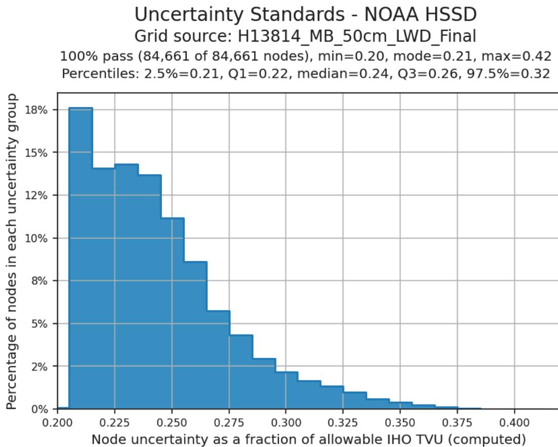
Figure 6: Uncertainty standards, 50cm resolution object detection coverage.
