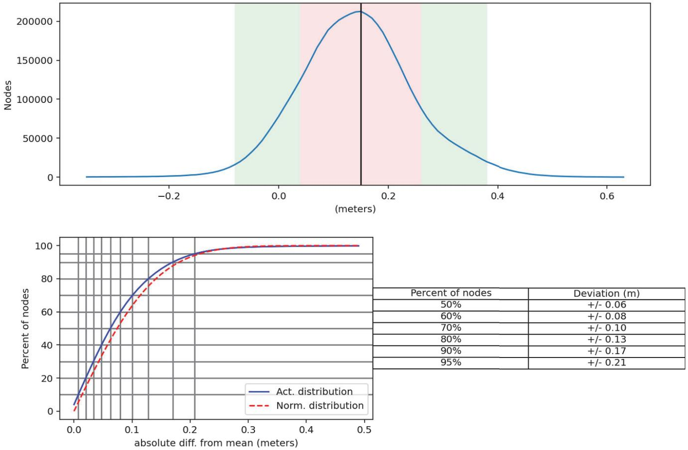
Figure 10: Depth differences between H13814 and bathymetric lidar data.
