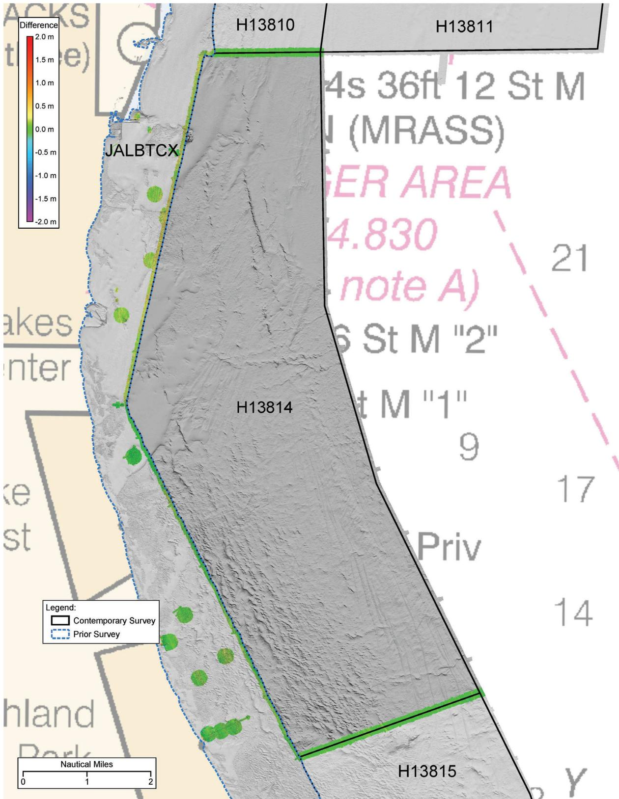
Figure 9: H13814 junction map with junction area depth differences.
