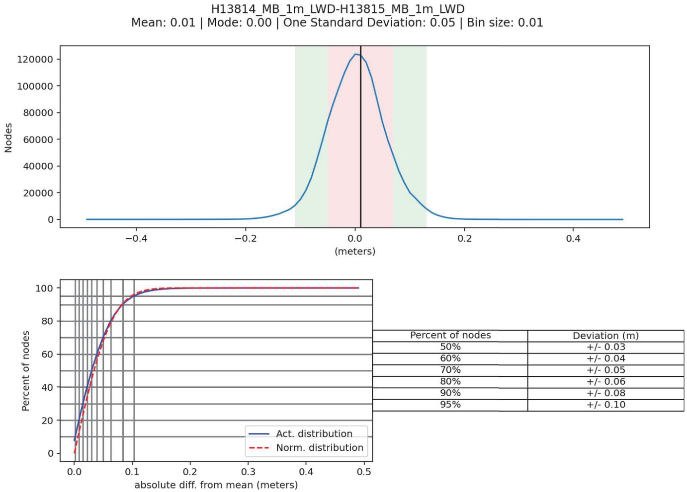
Figure 11: Depth differences between surveys H13814 and H13815.
