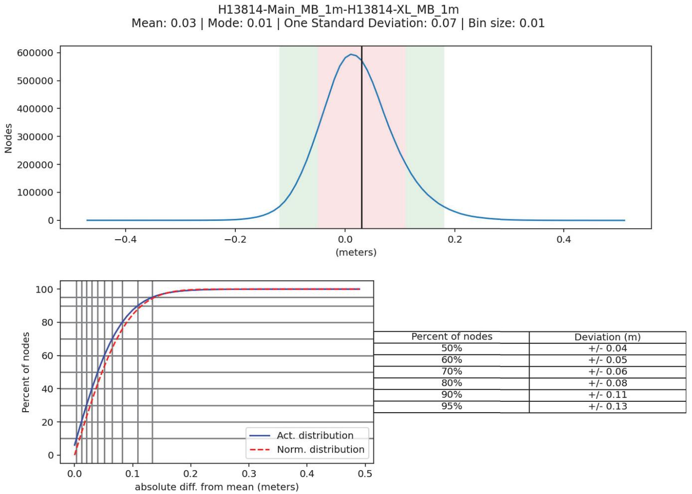
Figure 5: Depth differences between mainscheme and crossline data.
