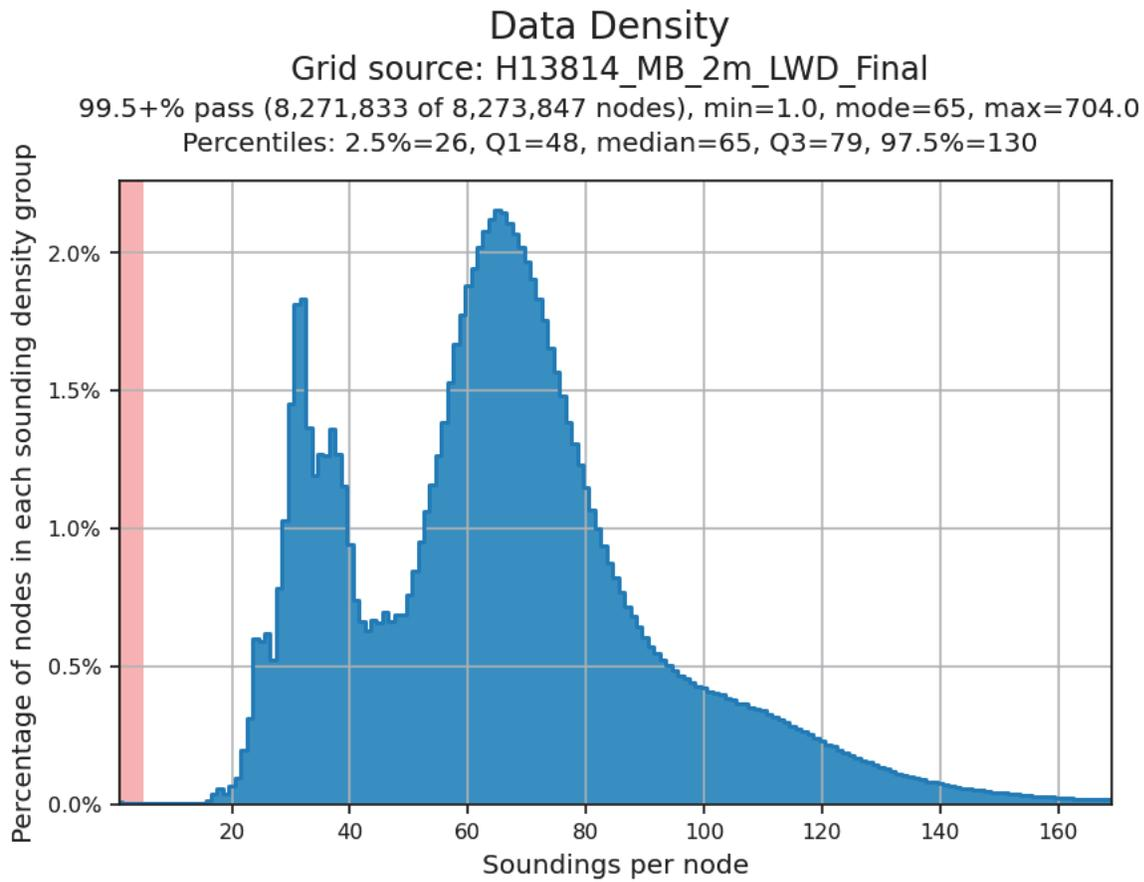
*Figure 15: Data density, 2m resolution complete coverage.*
