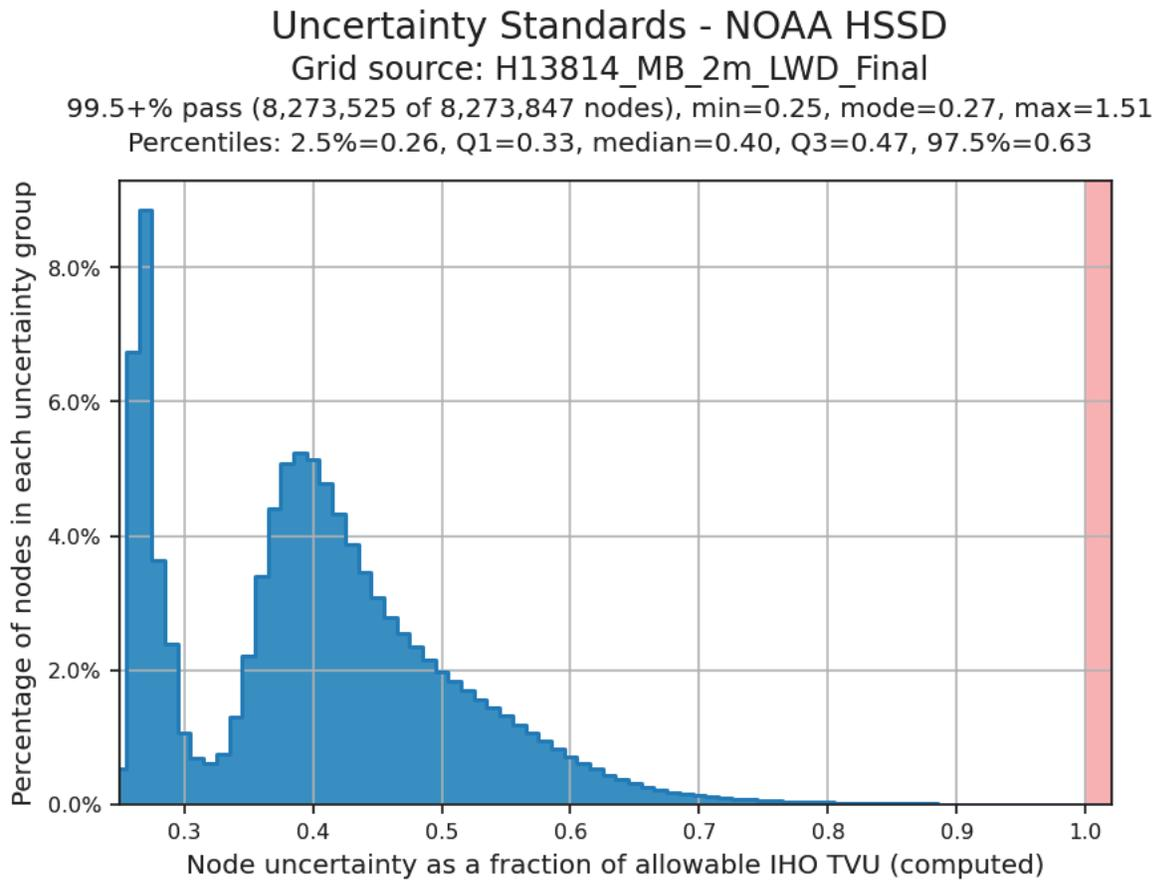
*Figure 8: Uncertainty standards, 2m resolution complete coverage.*
