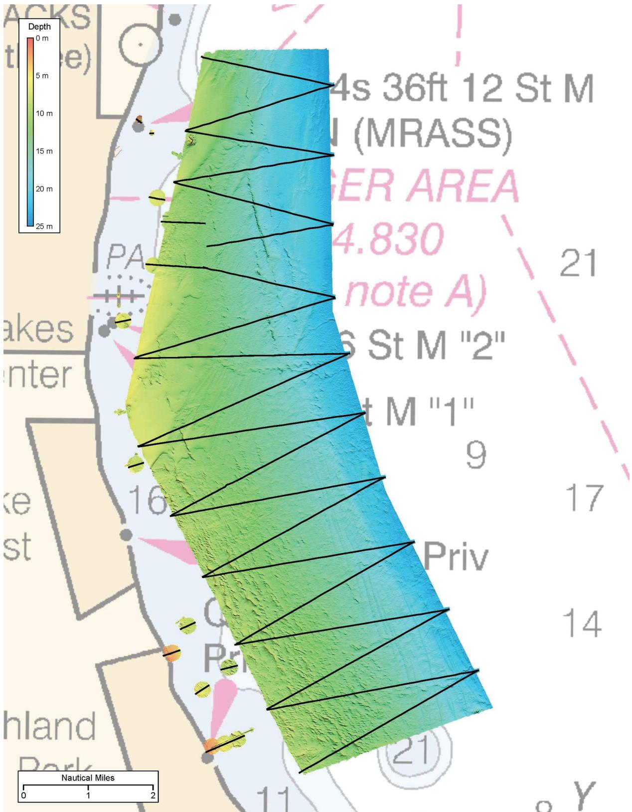
Figure 4: Crossline tracks overlaid on a coverage surface.
