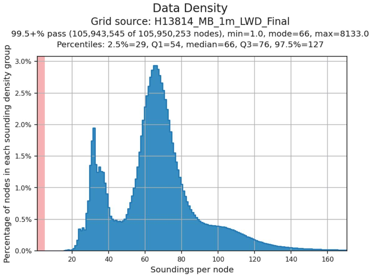
*Figure 14: Data density, 1m resolution complete coverage.*
