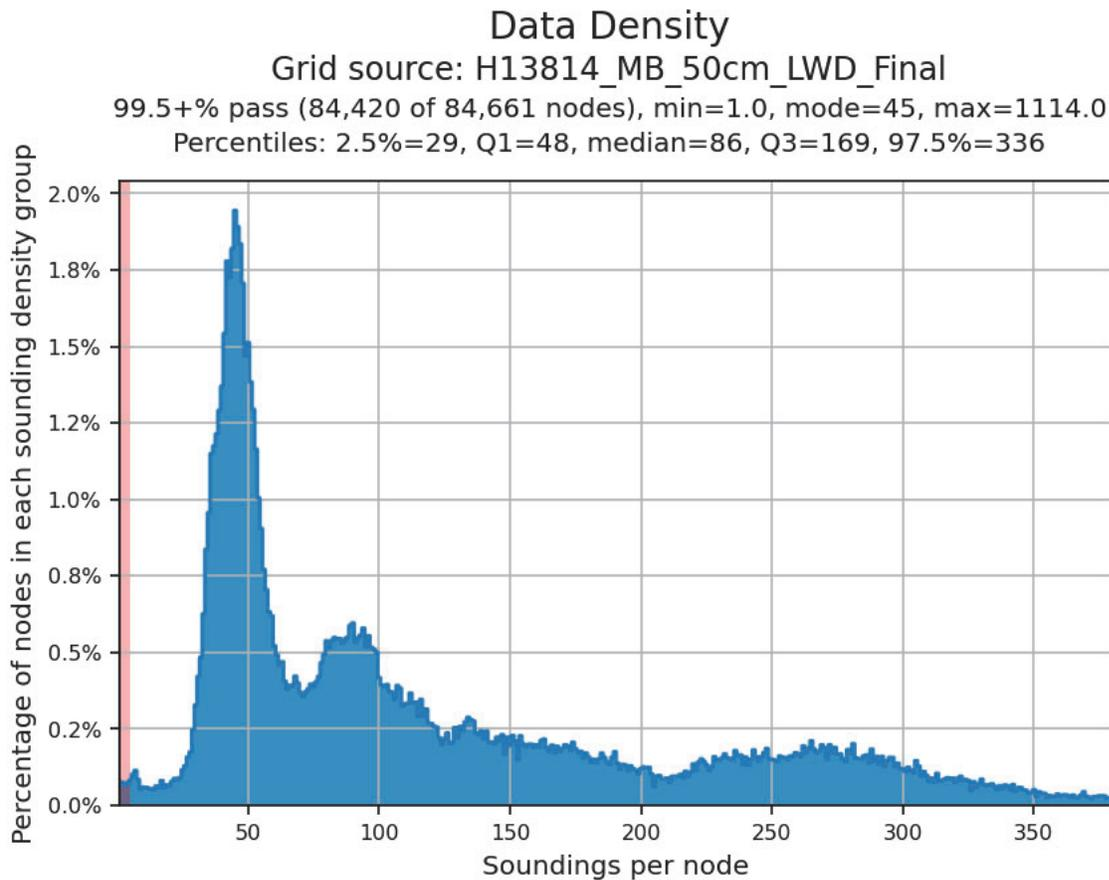
Figure 13: Data density, 50cm resolution object detection coverage.
