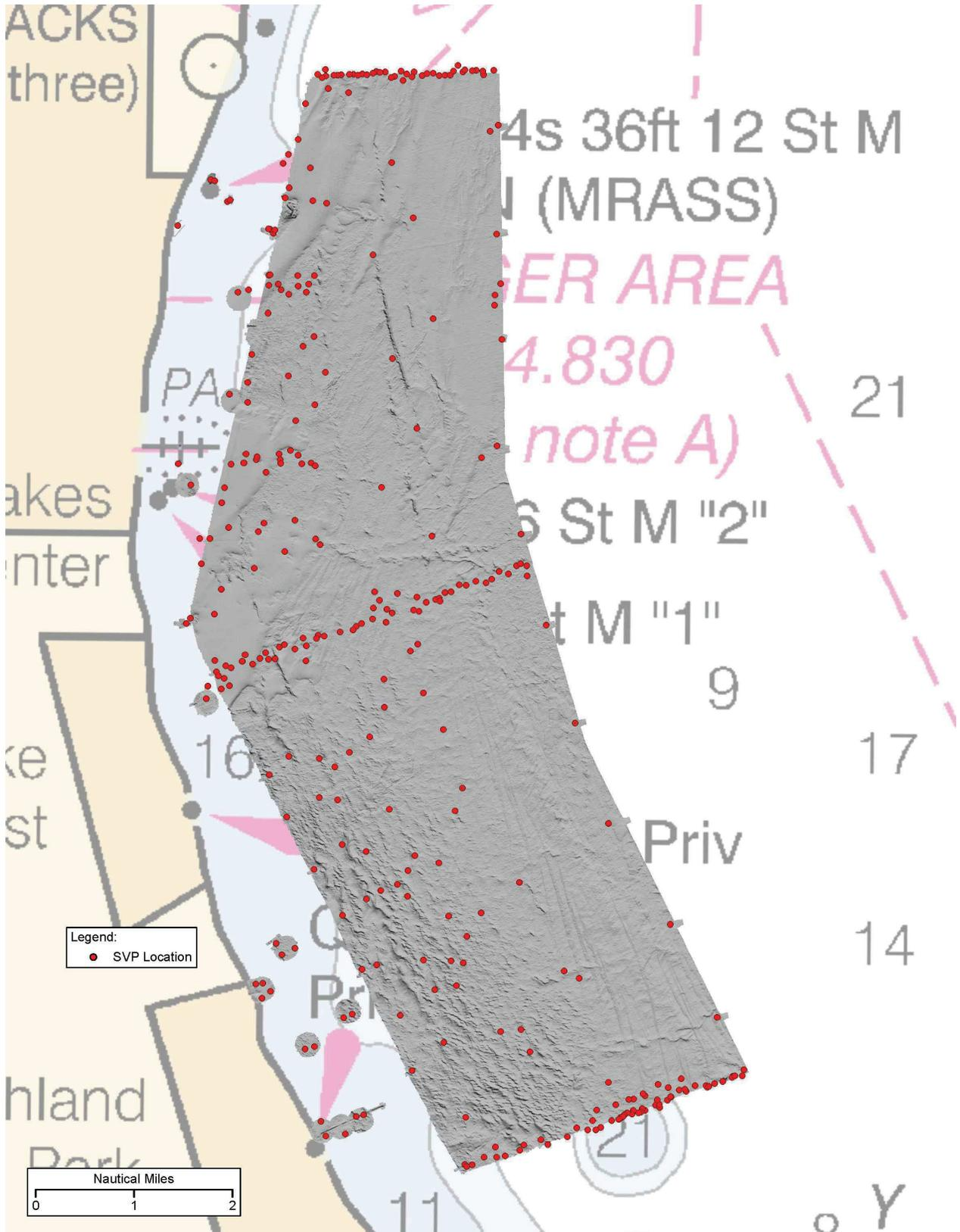
Figure 12: H13814 sound speed cast locations.
