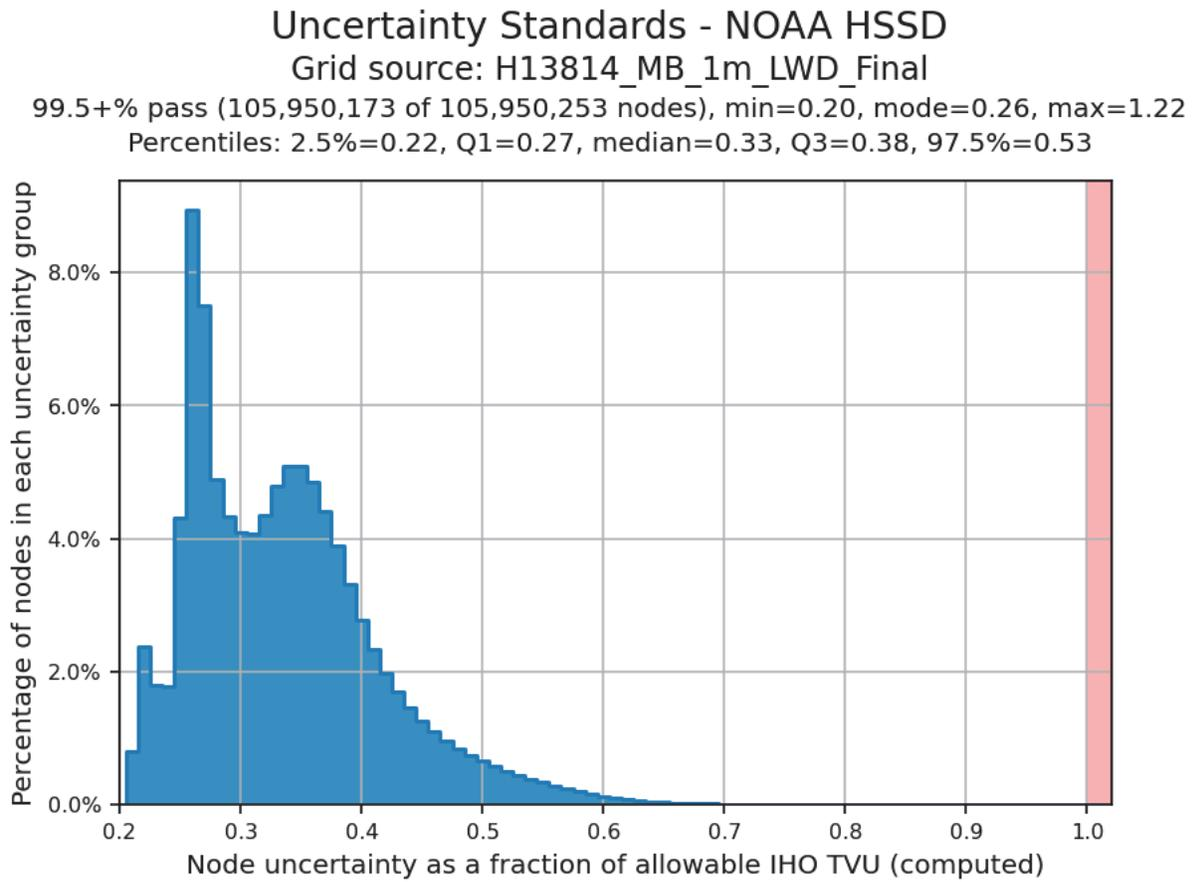
*Figure 7: Uncertainty standards, 1m resolution complete coverage.*
