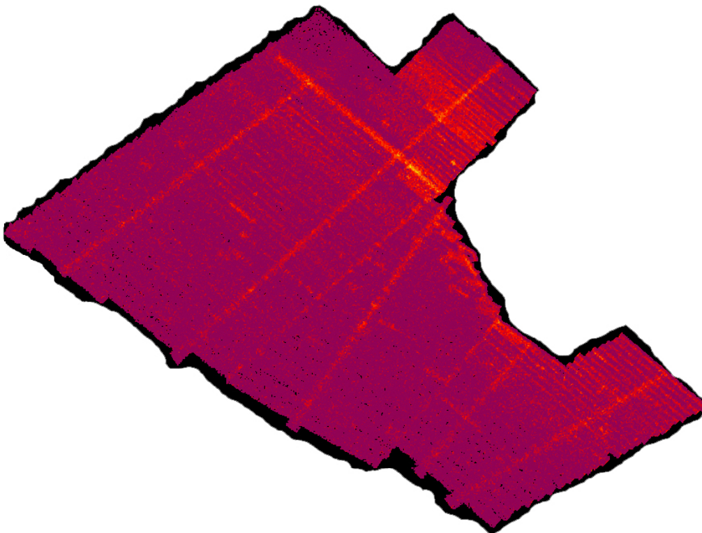
Figure 3. 5m density grid (magenta areas = 1 or 2 sounding contributing to the node)
