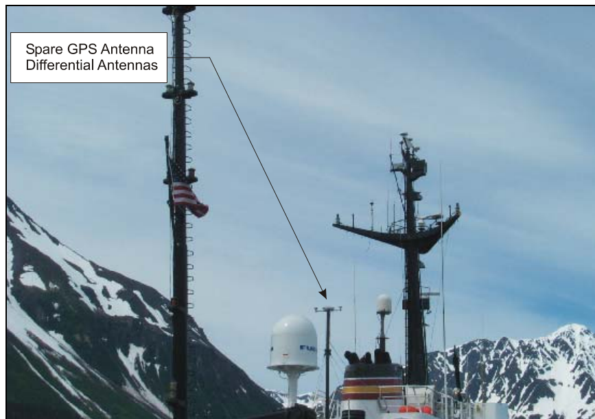
Figure B-4-2 Spare GPS and Differential Antennas
