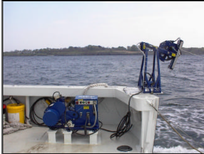
Figure 6. MVP Installation on the R/V OceanExplorer
