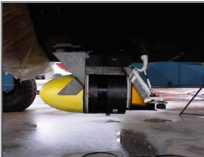
Figure 3. Reson 8101 Installation on the R/V OceanExplorer
