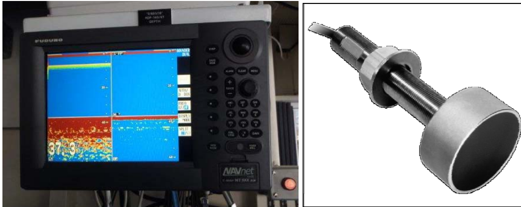
Figure 8: Furuno RDP 149/1934C plotter (S/N 4323-3869) left and Furuno 520-5MSD transducer (S/N Unknown) right
