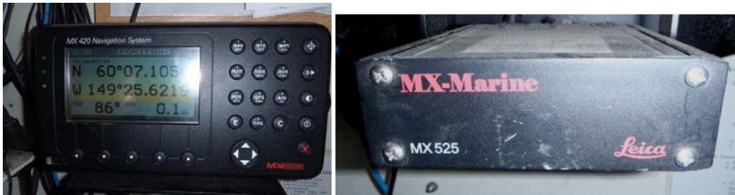
Figure 5: MX420 GPS receiver left (S/N 00805337) and MX-525 DGPS receiver right (S/N 0340-13002-0114)
