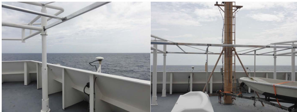
Figure 3. POS MV antenna position relative to ship superstructures.
