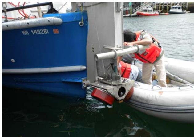
Figure 4 - EM3002 sonar heads mounted on the RV Coastal Surveyor
