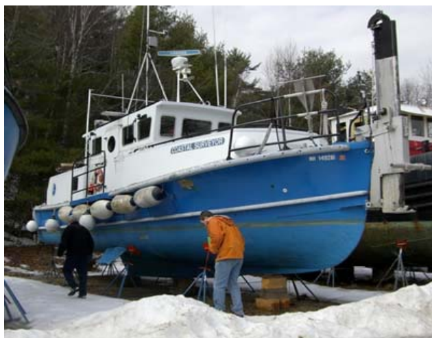
Figure 3 - RV Coastal Surveyor with bow ram for multibeam installation
