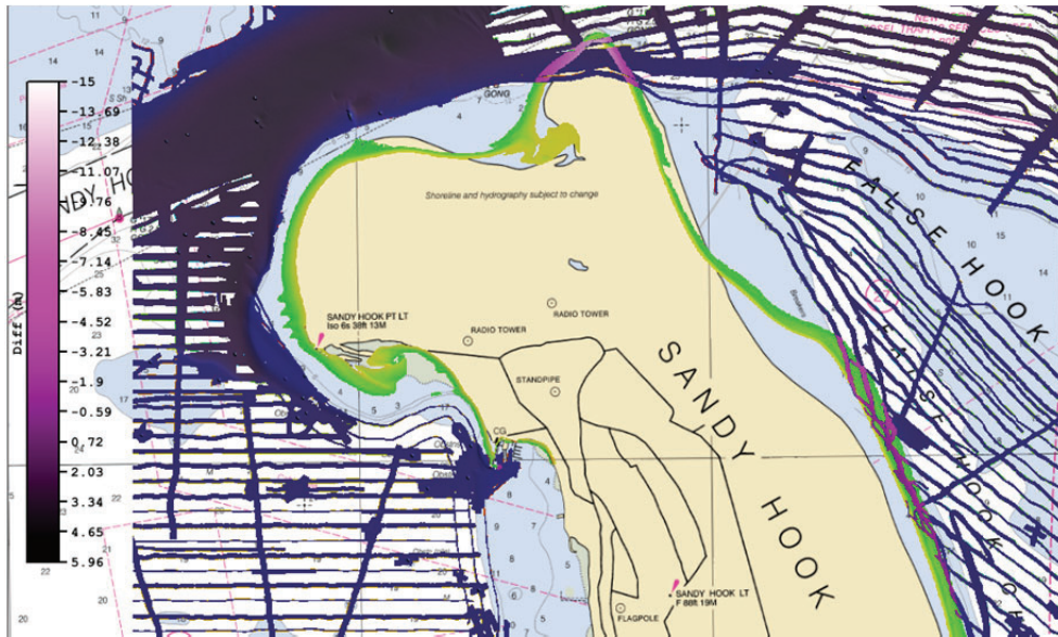
Figure 7 Area of overlap (magenta) between survey H11709 (blue) and W00302 (green) at Sandy Hook. W00302 was found on average 5.62 m shoaler, due to the changing morphology of the point over the seven year period between surveys. Background chart 12401, 1:15,000.
