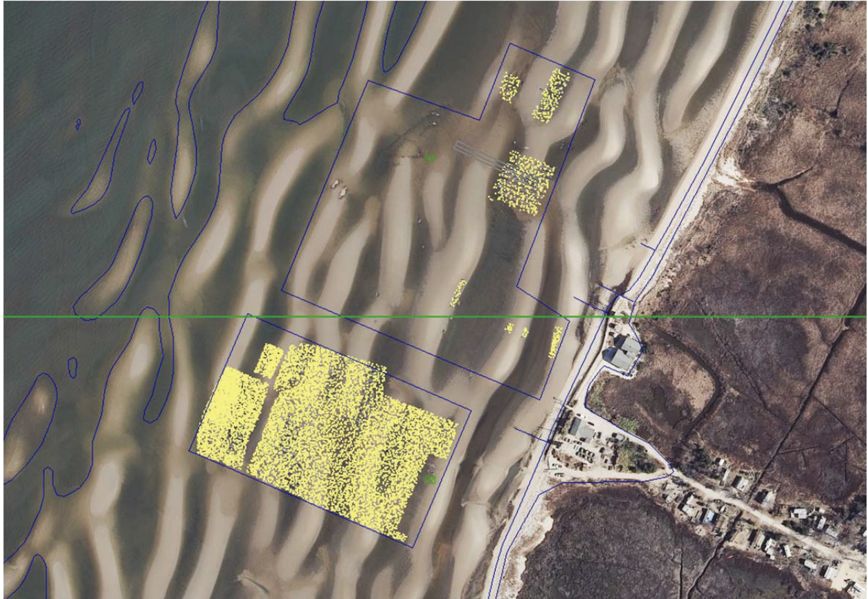
Figure 2 Class 30 lidar points (yellow) representing aquaculture facility between blocks 97 and 98. Green line represents border between blocks. These features were delineated in the RSD shoreline GC11175 (blue lines).
