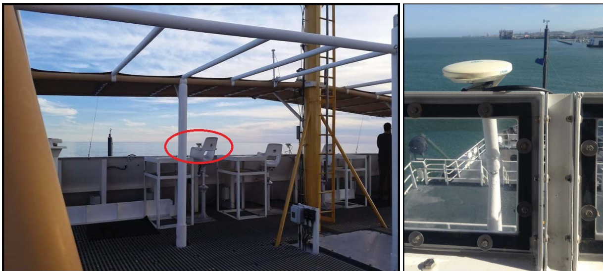
Figure 6: Location of POS antenna on the flying bridge (2015) & added plexiglass windshield (2016)
