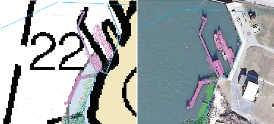
Figure 10 Unclassified lidar points (pink) detect pier not digitized in RSD shoreline (blue). Left: background Chart 12211 inset, 1:20,000.
