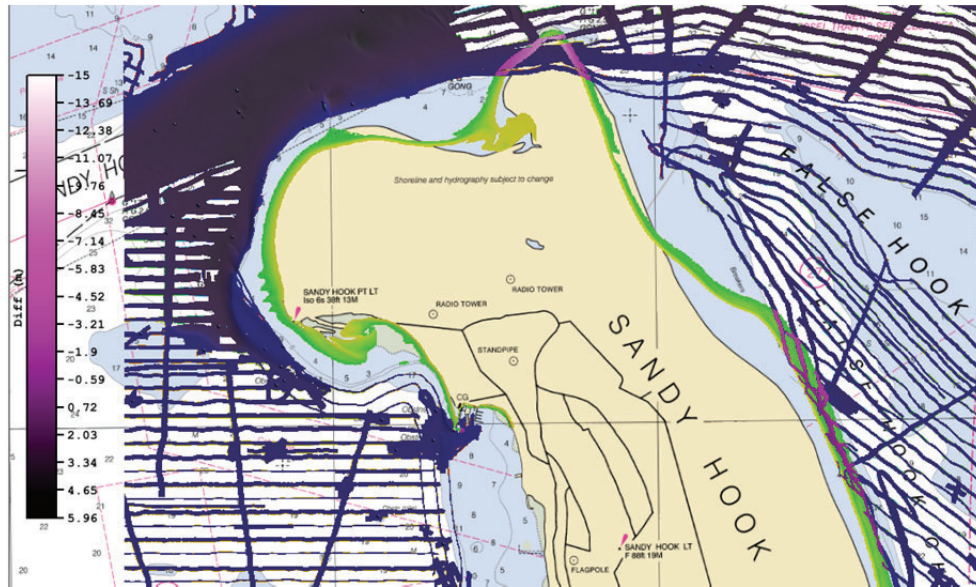
Figure 7 Area of overlap (magenta) between survey H11709 (blue) and W00300 (green) at Sandy Hook. W00302 was found on average 5.62 m shoaler, due to the changing morphology of the point over the seven year period between surveys. Background chart 12401, 1:15,000.
