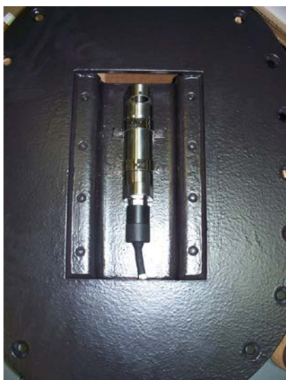
Figure 13. Photo showing the Reson SVP-70 probe attached to the access cover on the hull.
