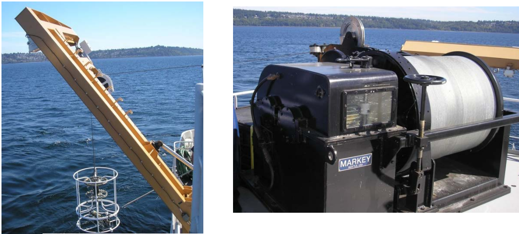
Figure 1. Photos of starboard side CTD deck showing J-Frame (left) and CTD Winch (right).
