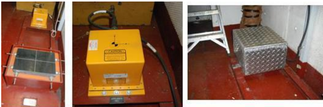
Figure 7. Photos: Clockwise from top left: IMU and granite block, IMU, IMU under protective housing.
