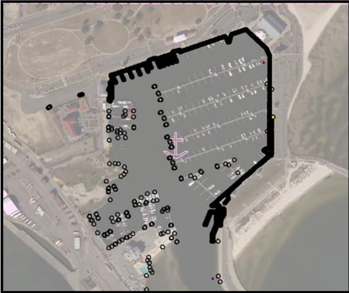
Figure 32. RTK data overlaid on aerial photogrammetry.
