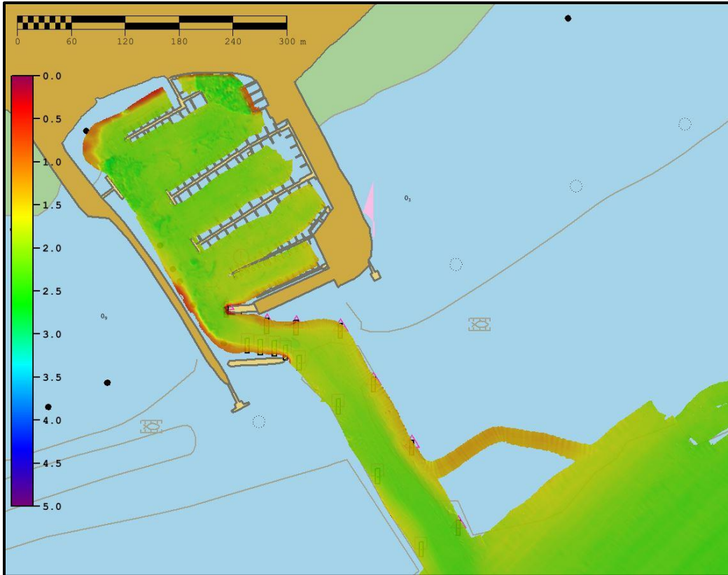
Figure 4. EdgeTech bathymetry coverage within the harbor with colored depth in meters.
