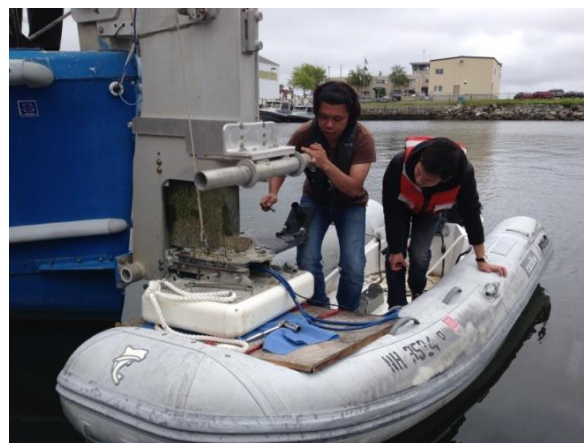
Figure 1: R/V Coastal Surveyor Adjustable bow ram with winch and transducer mount.
