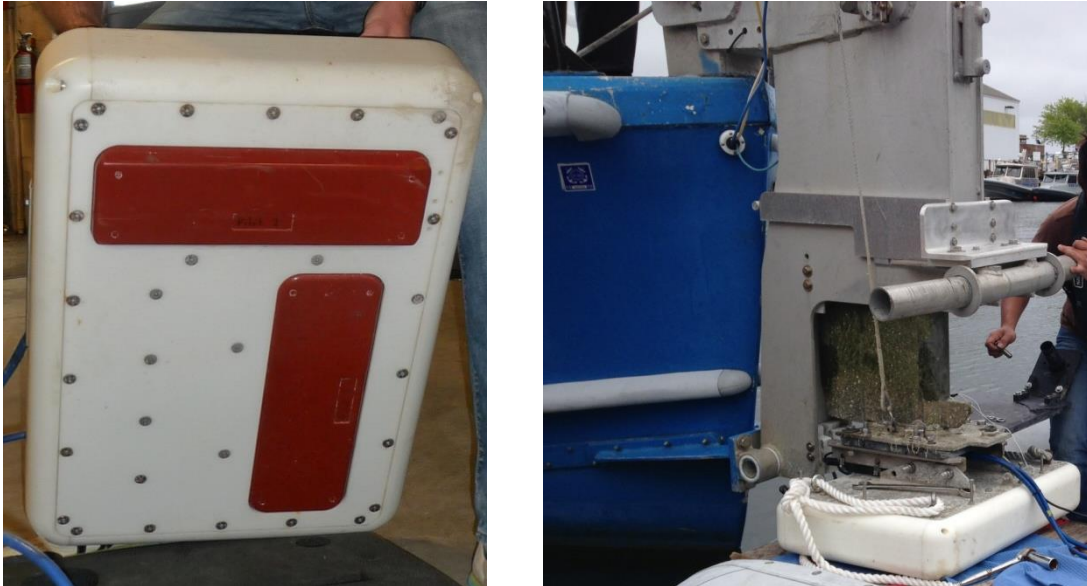
Figure 3: - EM 2040 Transducer Face (left) and how it is mounted (right).
