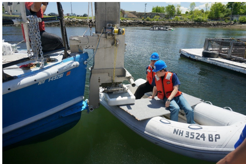
Figure 6: Kongsberg EM 2040 transducer installed on bow mount of R/V Coastal Surveyor
