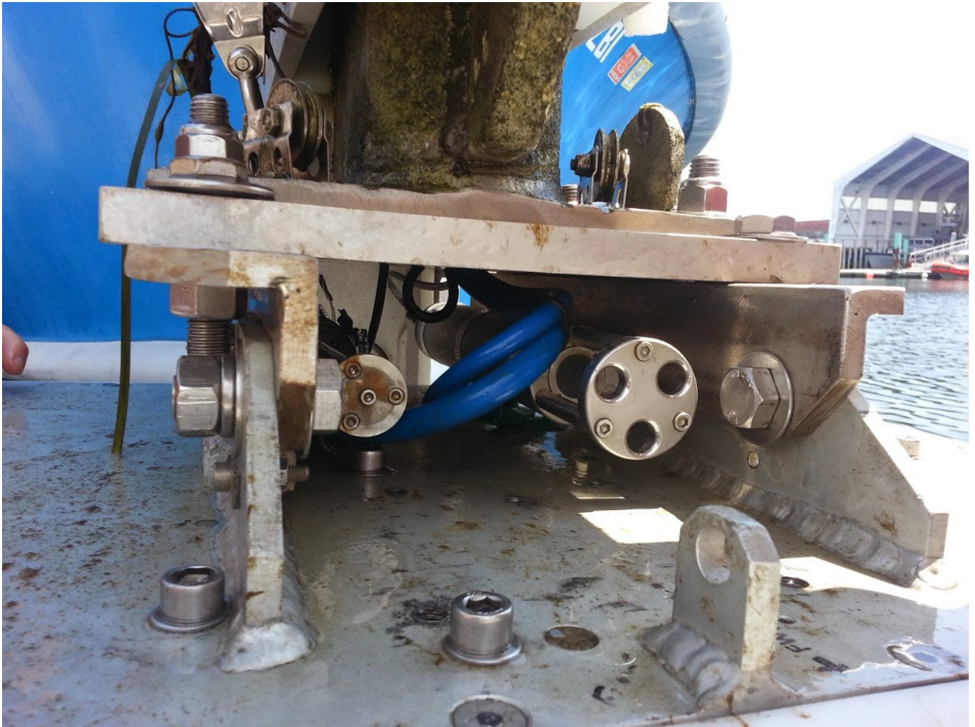
Figure 9: Digibar Pro (right) mounted on top of multibeam EM 2040 transducer
