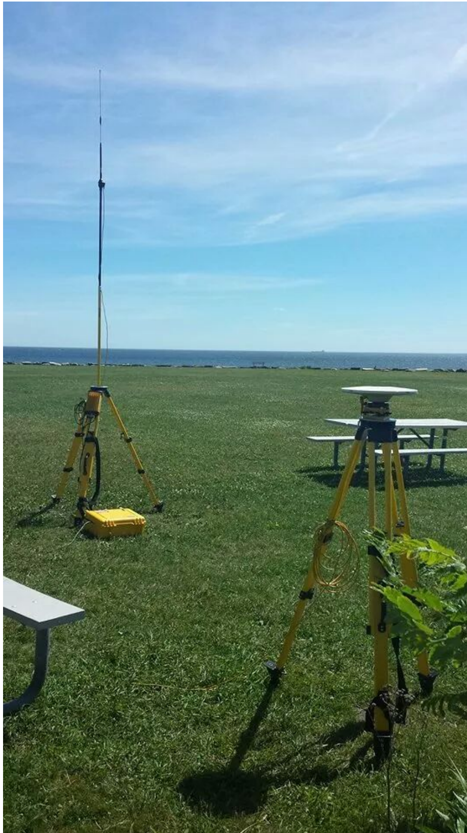
Figure 14: RTK base station at Rye Harbor State Park
