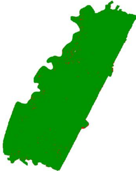
Figure 17. Overview of the density analysis surface. Green => 5 sounding per cell, Red < 5 sounding per cell.
