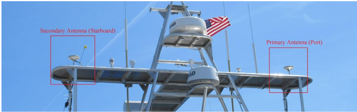
Figure 4. Applanix POS/MV antenna configuration.
