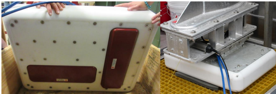
Figure 2. Kongsberg EM2040 multibeam echo sounder.
