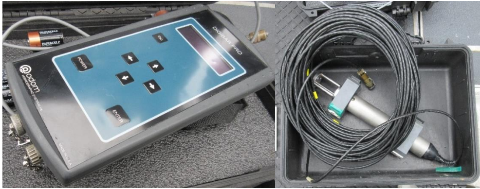
Figure 5. Odom Digibar Pro sound speed profiler.
