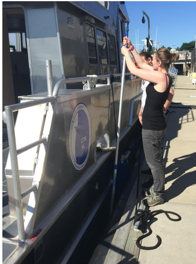
Figure 3. Boat hook measurement of water level at dock.
