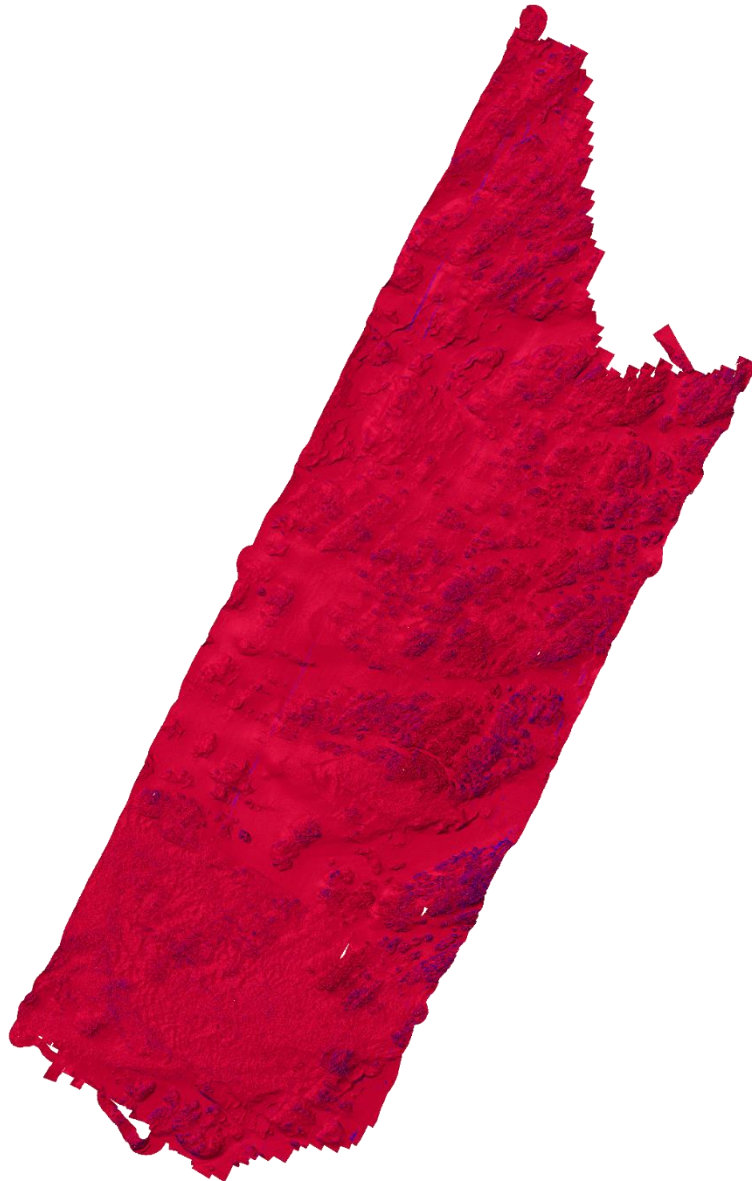
Figure 7: CUBE surface colored by uncertainty values. Values below 0.3m are in red (within Special Order Maximum Uncertainty).
