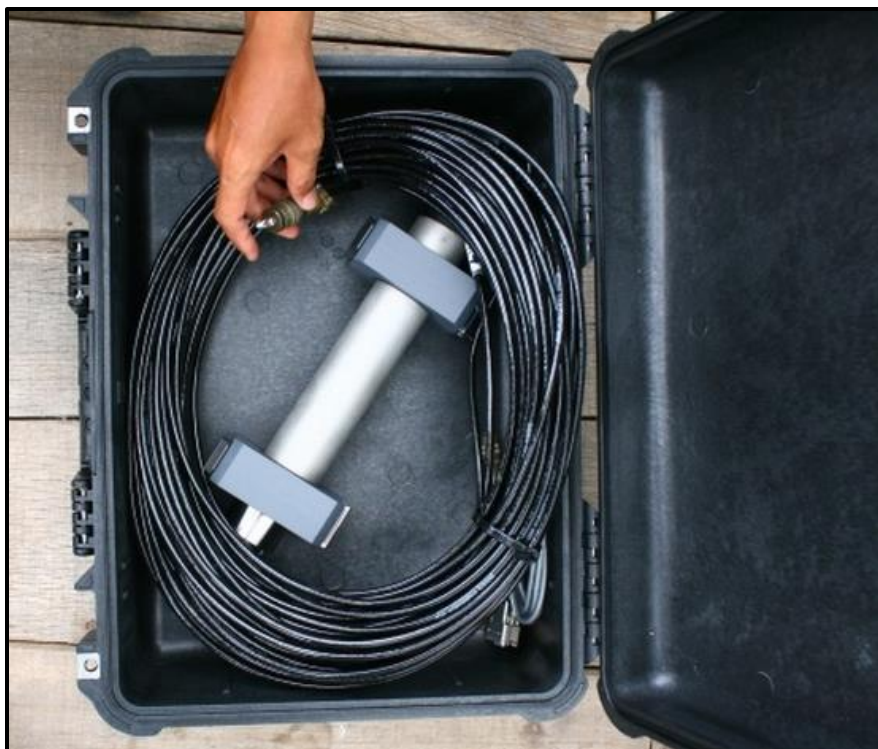
Figure 9: Odom Digibar sound speed probe
