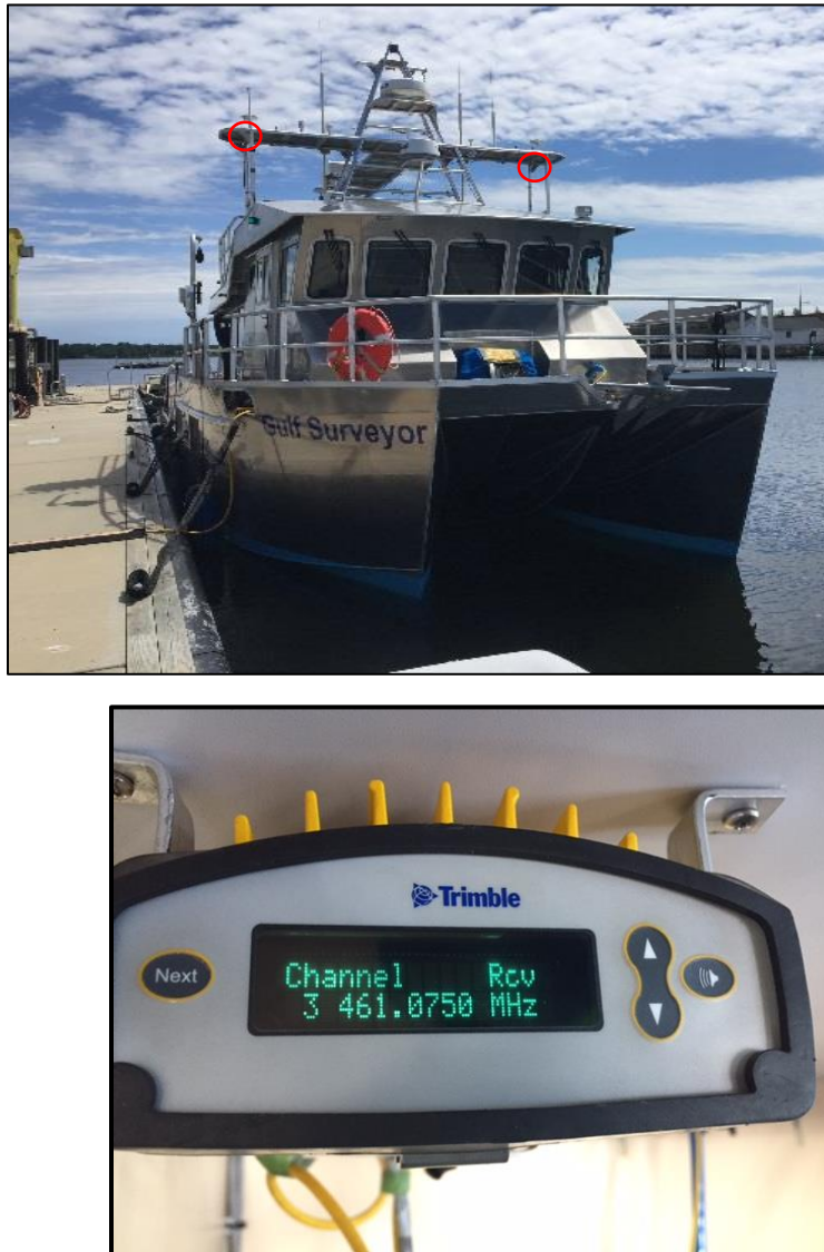
Figure 11: (top) GPS antennas (red circles) on RVGS top platform. (bottom) Trimble Receiver Modem inside main cabin above system rack.
