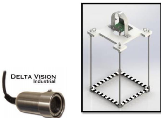
Figure 13: Drop camera cage (right) and camera (left)
