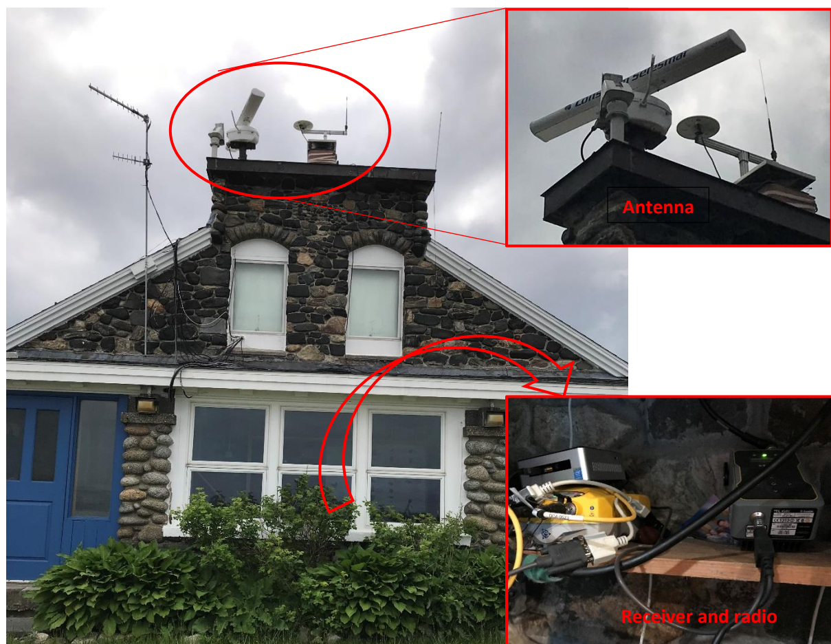
Figure 2. Instrumentation of the RTK Base Station at the Seacoast Science Center, Odiorne Park, Rye, NH.
