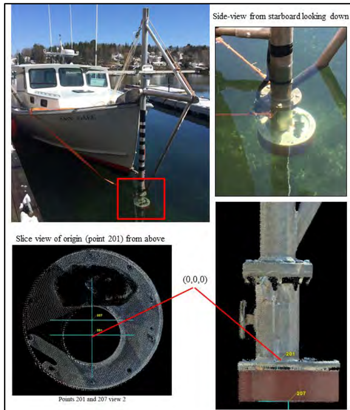
Figure 8 – Amy Gale origin (point 201 in RGB images) for vessel reference frame(s); origin is center point within the base of the pole (center point of base within internally-mounted motion reference unit (MRU) point 201 in images above)
