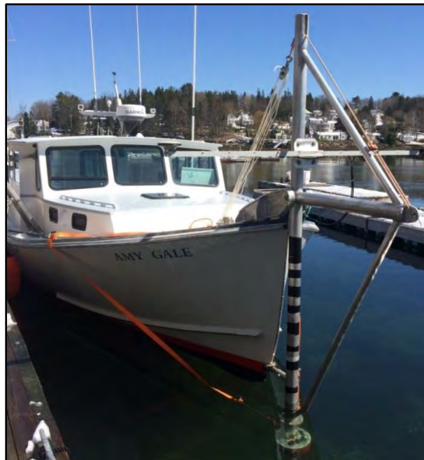
Figure 6 – R/V Amy Gale shown with pole-mounted dual GPS antennas, Kongsberg EM2040C multibeam sonar, MRU (not visible), and surface sound speed probe (not visible) in acquisition mode
