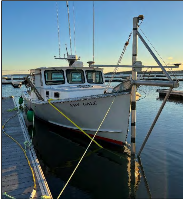
Figure 4 – F/V Amy Gale shown with pole-mounted dual GPS antennas, Fugro AD-341 antenna, Kongsberg EM2040C multibeam sonar (not visible), MRU (not visible), and surface sound speed probe (not visible) in acquisition mode.
