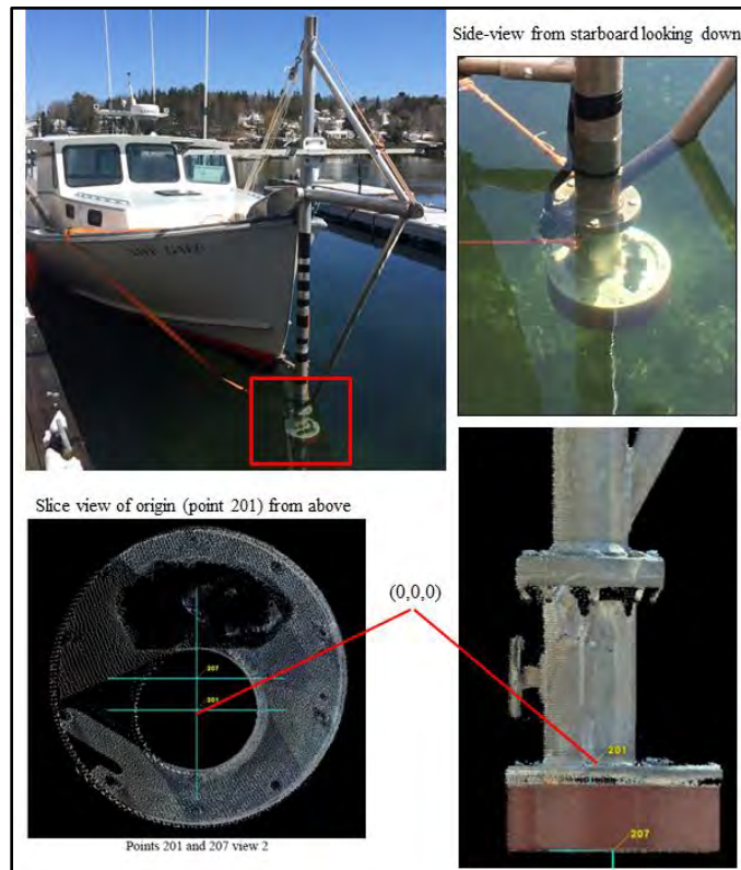
Figure 6 – Amy Gale origin (point 201 in RGB images) for vessel reference frame(s); origin is center point within the base of the pole (center point of base within internally-mounted motion reference unit (MRU) point 201 in images above)
