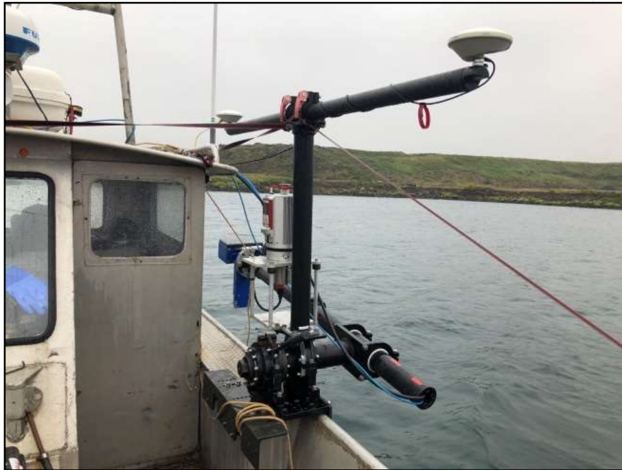
Figure 4 eTrac VOOP with mounted with R2Sonic 2022 & Riegl VZ-400
