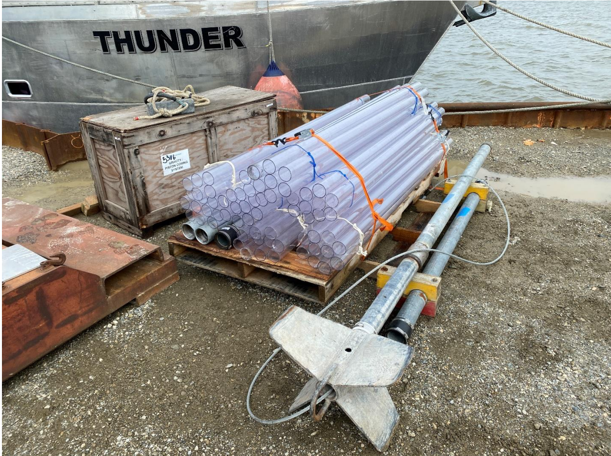
Figure 2-3. Piston Core and core liners ready for mobilization.
