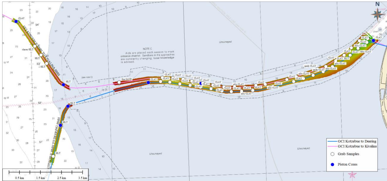
Figure 5-13. Zone 1 Geotech stations
