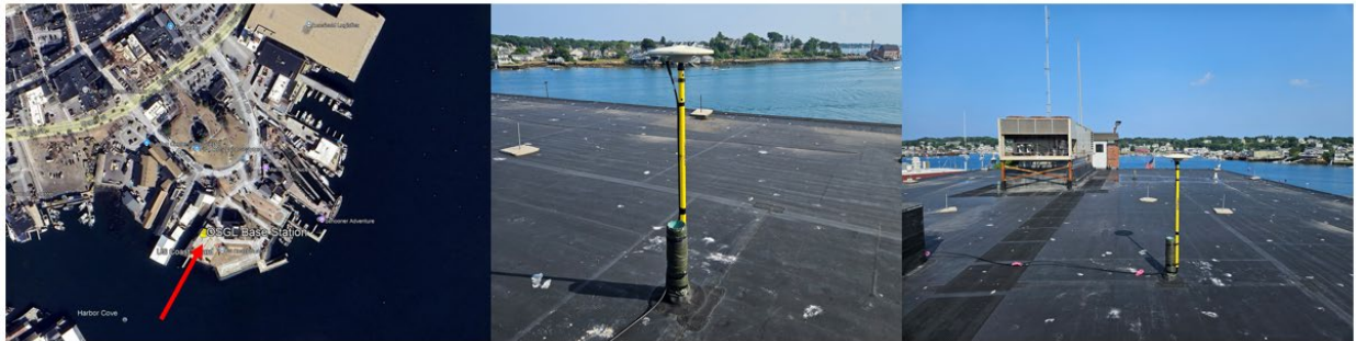
Figure 3. Ortho imagery and setup images of OSI’s user-installed base station “OSGL” on the roof of US Coast Guard Station Gloucester in Gloucester, Massachusetts.
