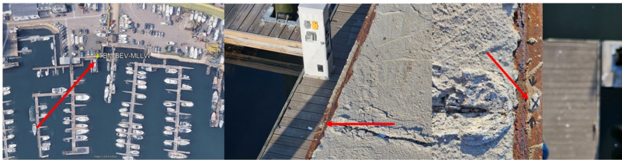
Figure 6. “TBM BEV-MLLW” is a black X in a noticeable divot at the top of the bulkhead at Beverly Port Marina in Beverly, Massachusetts.
