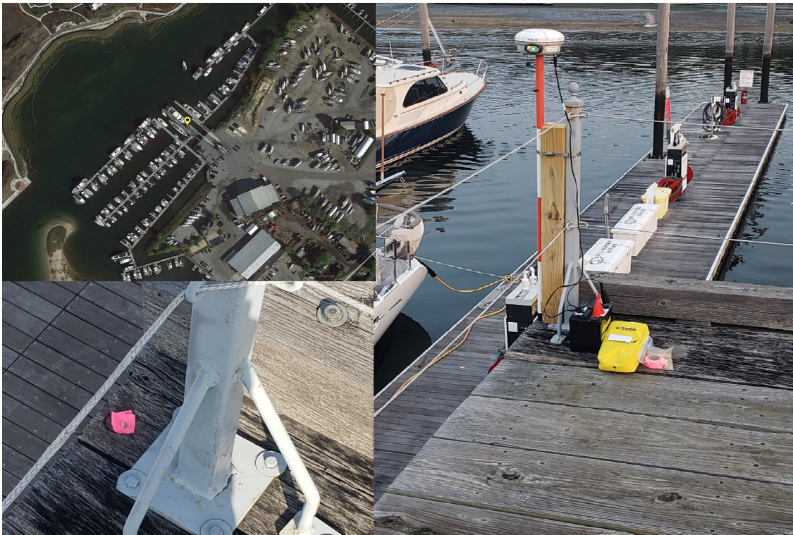
Figure 8. “GC20” is a pink flagged PK Nail in a dock at Glen Cove Marina in Glen Cove, NY.
