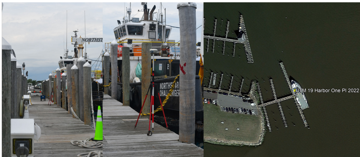
Figure 4. “UTM 19 Harbor One PI 2022” is a deck screw backed with yellow tape on pier decking at north half of Plum Island Crew Boat pier in Old Saybrook, CT.
