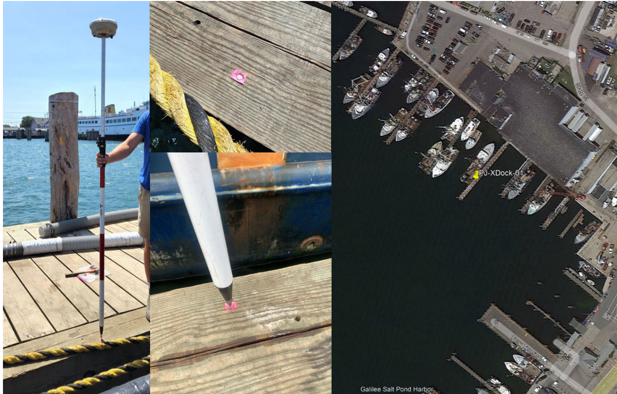
Figure 5. “PJ-XDock-01” is a pink backed PK nail in pier decking on the west side of X-Dock at Point Judith State Docks in Point Judith, RI.
