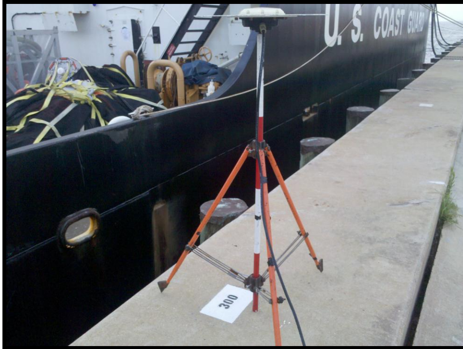
Figure 4. Acquiring position data at checkpoint “NAS Pier B Station 300” using the Trimble MS750 GPS.
