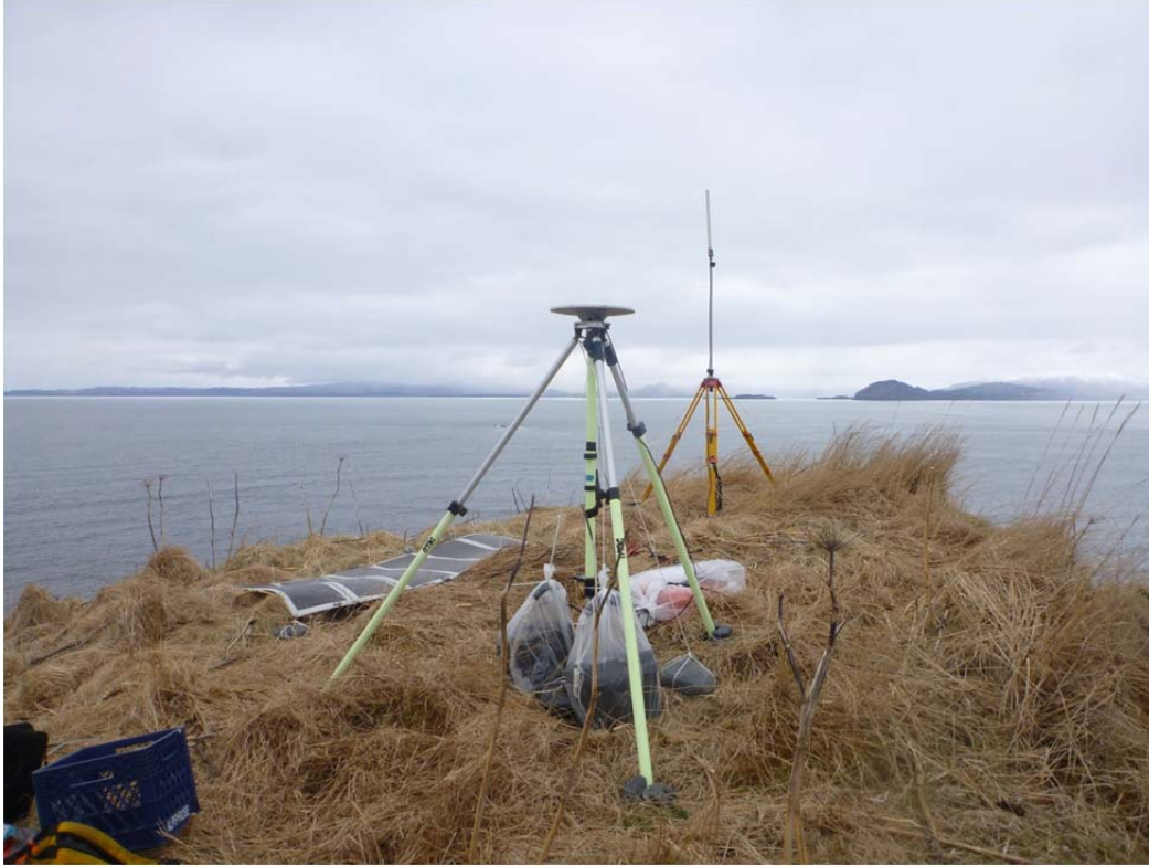
Figure 3: Woody GNSS Antenna and solar panel array.
