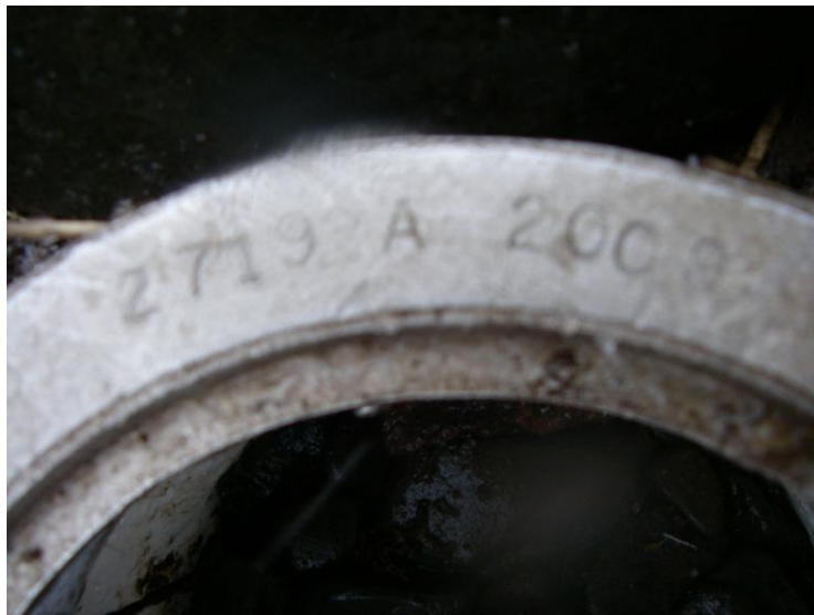
Figure 1 - Stamping of GPS benchmark 9462719 A
