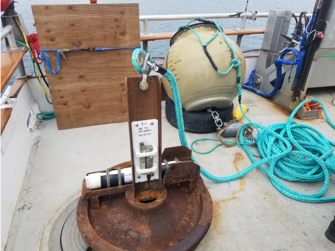
Figure 4 Ikatán Bay tide equipment prior to deployment: BMPG mooring and JOA GPS buoy
