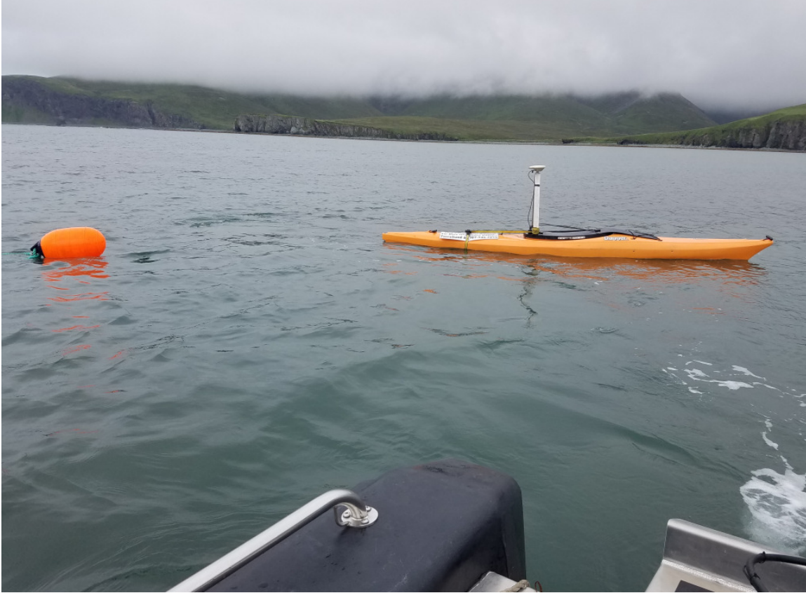
Figure 3 – GPS buoy kayak in Dora Harbor
