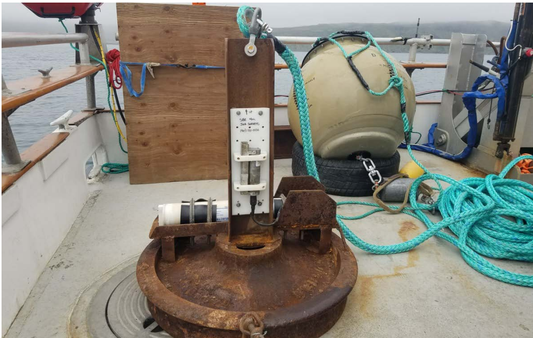
FIGURE 3 - PICTURE OF THE BMPG MOORING AND GPS BUOY DEPLOYED IN IKATAN BAY.
