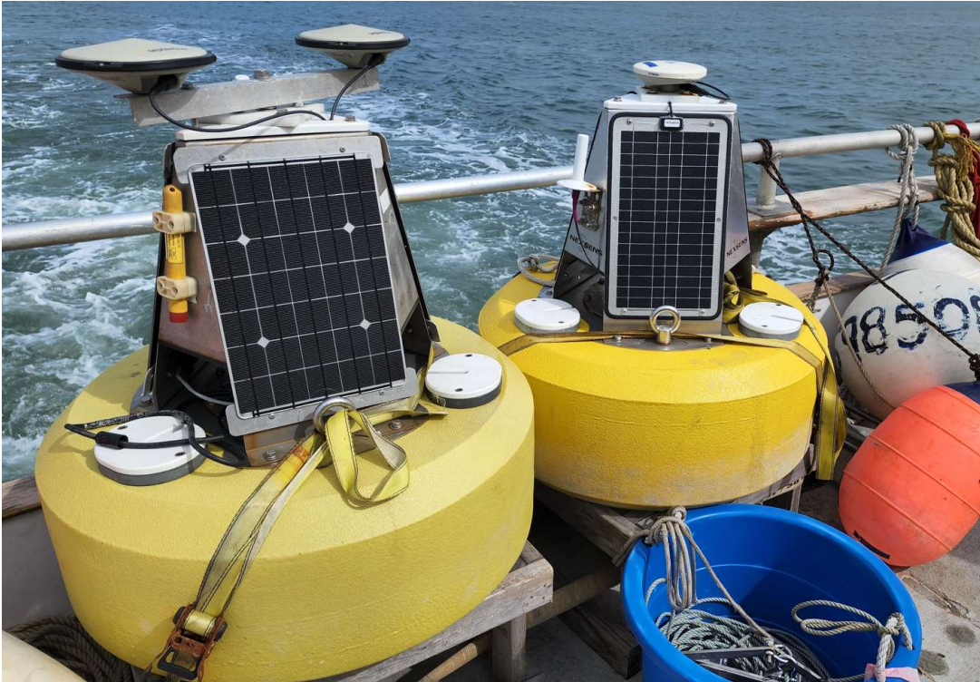
Figure 2 – The two project GNSS tide buoys after retrieval. The Southwest Nunivak buoy is on the left, while the Northwest Nunivak buoy is on the right.
