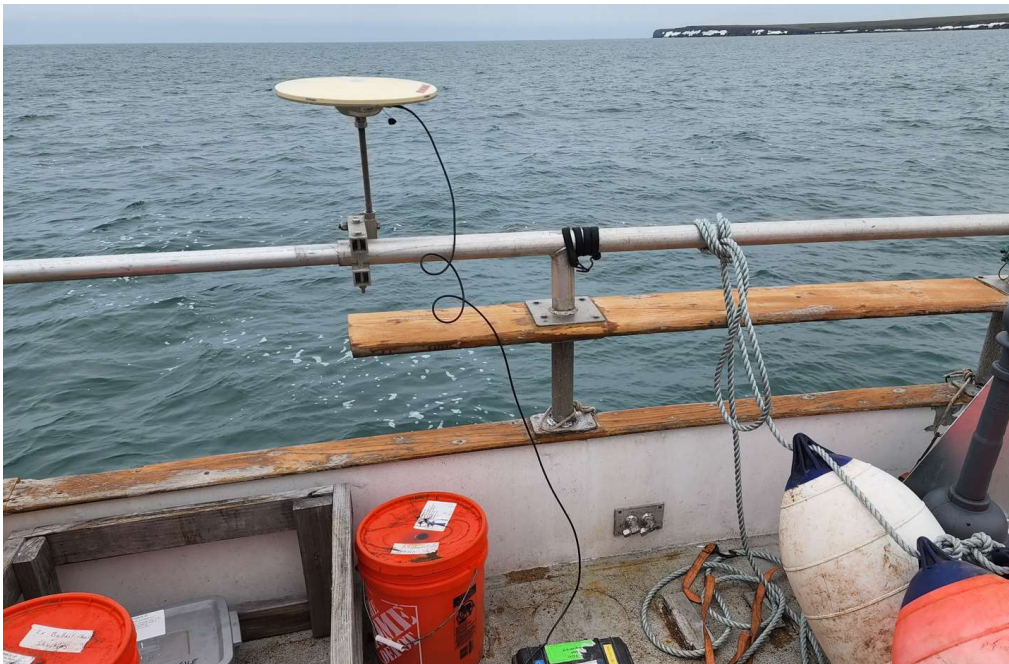
Figure 3 – Trimble 5700 GNSS antenna on the back deck of the survey vessel used for comparisons with the buoy data. Vessel POSMV data was also used.
