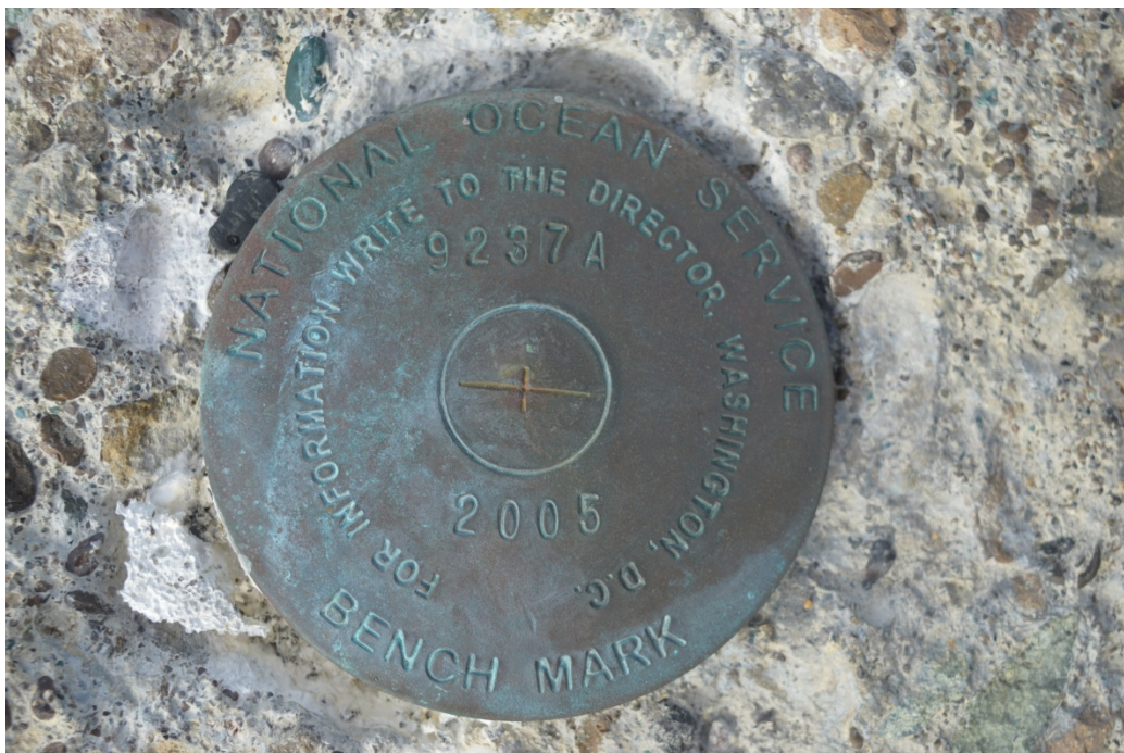
Figure 5, Installed horizontal control mark “9237A”
