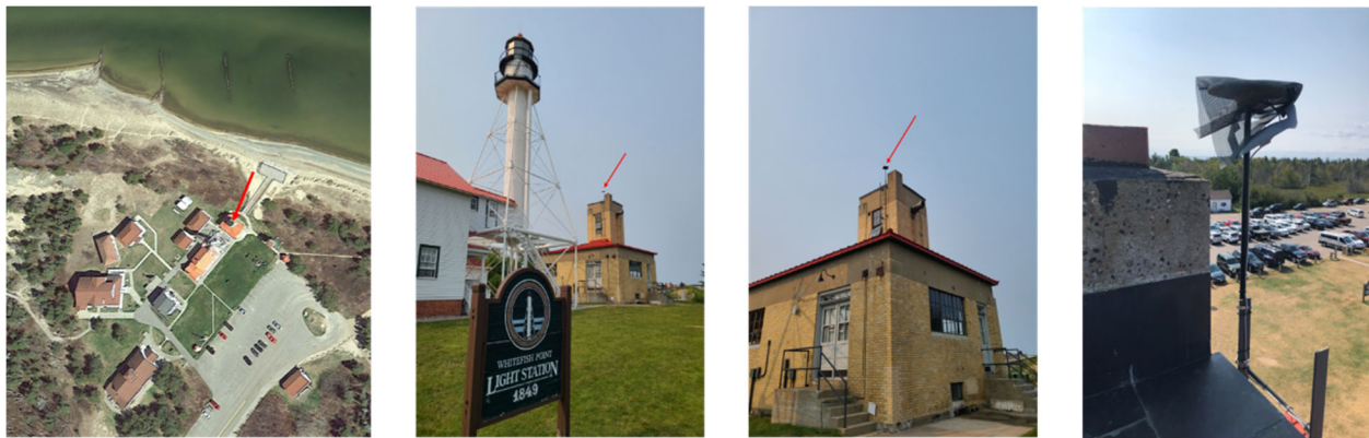
Figure 2. Ortho imagery and setup images of OSI’s user-installed base station “OSWP” on top of a building at the Great Lakes Shipwreck Museum in Paradise, MI. At the request of the museum, the GNSS antenna was camouflaged to preserve the historic character of the structure (far right panel).
