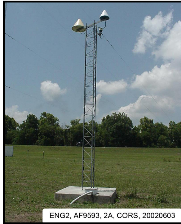
Figure 7 - Continuously Operating Reference Station (CORS) English Turn, LA
