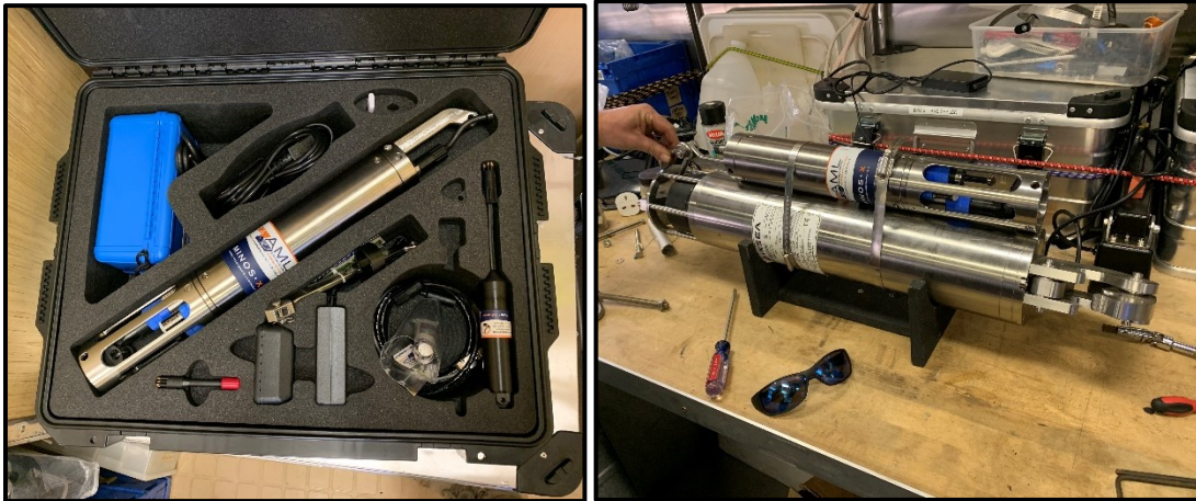
Figure 7: AML Minos-X SVP in box (left) and attached to the lander (right).
